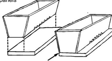
Mark out and cut triangular entrance holes 2.5cm wide by 2.5cm deep in the front panel, then nail the top to the base.
