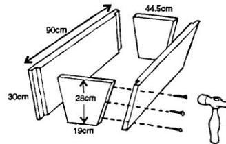
The ends of the front and rear panels are nailed to the side panels
