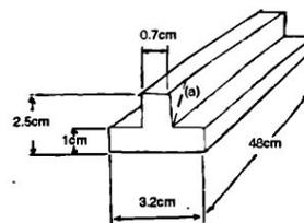
The top bars must be built accurately. You will need to cut 27 of them and the ends (a) must be shaped to the angle of the sides of the hive.
