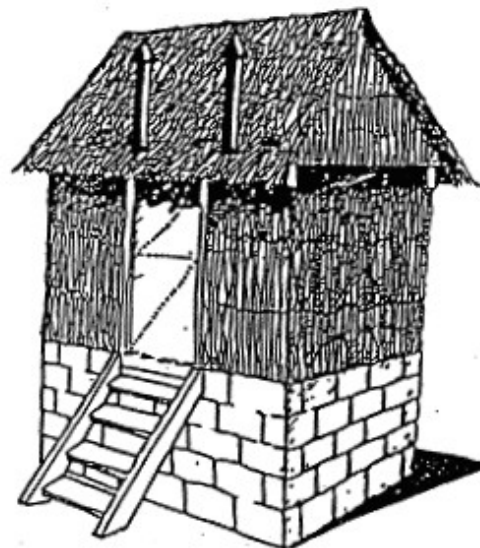
COMPLETED TOILET (Clad with local materials)
