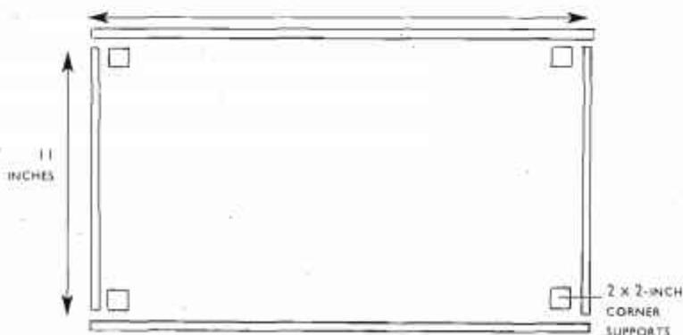
**DIAGRAM #2: EXPANDED TOP VIEW OF BIN AND CORNER SUPPORTS**
