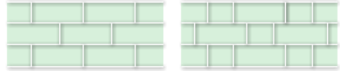
Typical brick patterns of cavity walls (left) and solid walls (right)
