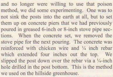
The pier method has a built-in flaw which we anticipated from the start. We call it "hinging". This is when the pressure from the earth behind the wall pushes in hard enough to push both the post and pier into the structure a bit, as in the illustration. To avoid this, the post must
