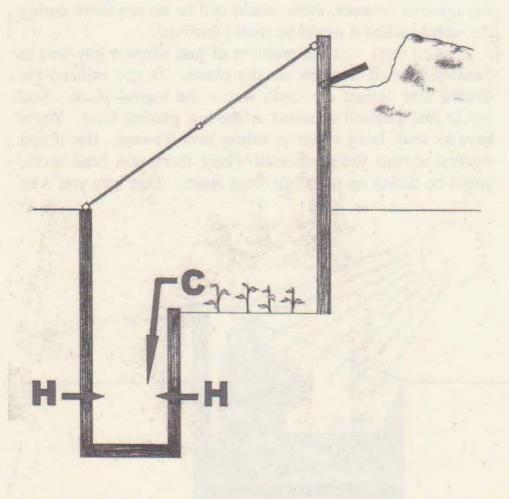
greenhouses four-season successes. The cold-sink concept is this, and it is this simple: The coldest air, which would sink to the otherwise lowest spot, the growing bed, now spills into the trench where it is warmed by the earth behind the walls.
