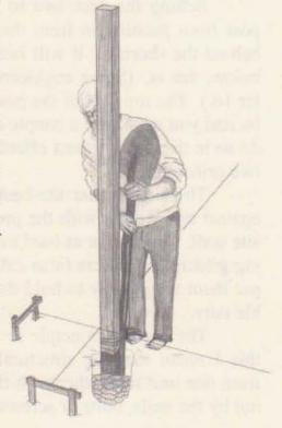
sprinkle on water and mix it up as though we were mixing concrete – though nowhere near that moist. Trial and error will show you the right moisture content for solid tamping in your particular soils.
