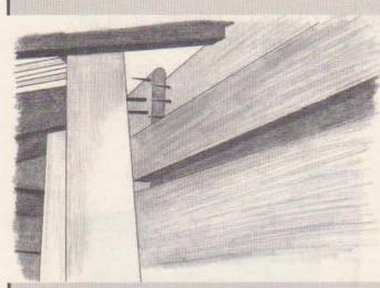
with the joints in the glazing. So some of the posts did not have the direct bone support advantage of the rafters. We put the girder board, which spans between the posts of which some of the rafters are notched into, on the outside of the posts instead of inside. The rafters notched into
