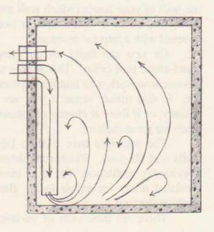
take care to provide ventilation. The illustration on the previous page shows one example. The principle is cool air comes in below and warmer air exits above.
