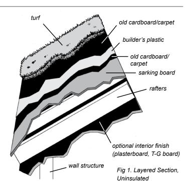
t by at least 500mm such that the water will flow away from the overlap. If this is impossible to do, for example because of the shape of the roof, then it would probably be best to consider some other waterproofing layer. Having said that, DPM can be stuck together with cold tar or lap cement and this is worth considering, even if it is a calculated risk. Edge details are best done like conventional flat roofs.
