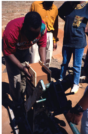
Figure 2: Brick moulding, Zimbabwe ©Practical Action/Theo Schilderman
