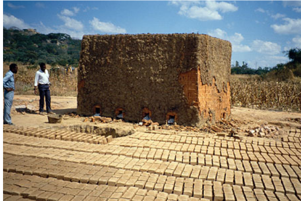
Figure 3: Coal fired bricks drying in sun Zimbabwe ©Practical Action/Theo Schilderman
