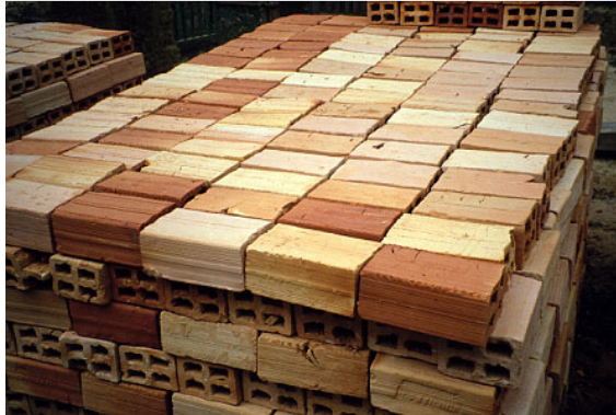
Figure 1: A pile of fired bricks, Alto Mayo, Peru. To be noted are the cracks and deficiencies in the bricks. ©Practical Action/Theo Schilderman
