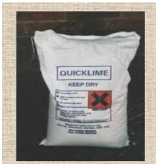
quicklime is different from ordinary 'bag lime' that you buy from a builder's merchants. It is calcium carbonate (limestone or chalk) which is burnt, driving off CO2 to leave calcium oxide.
