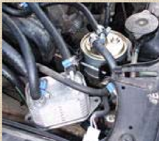
'Elsbett' engine conversion: filter heater and heat exchanger mounted in car.
