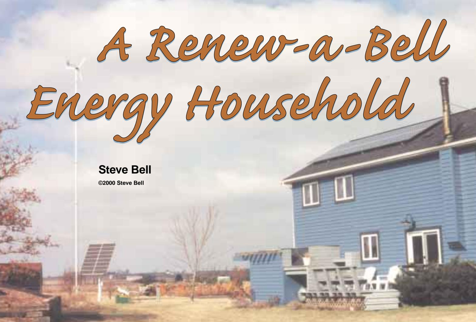
Steve and Jan Bell's home with 2,100 watts of roof-mounted PV, 880 watts of tracked PV, and 3,600 watts of wind power.
