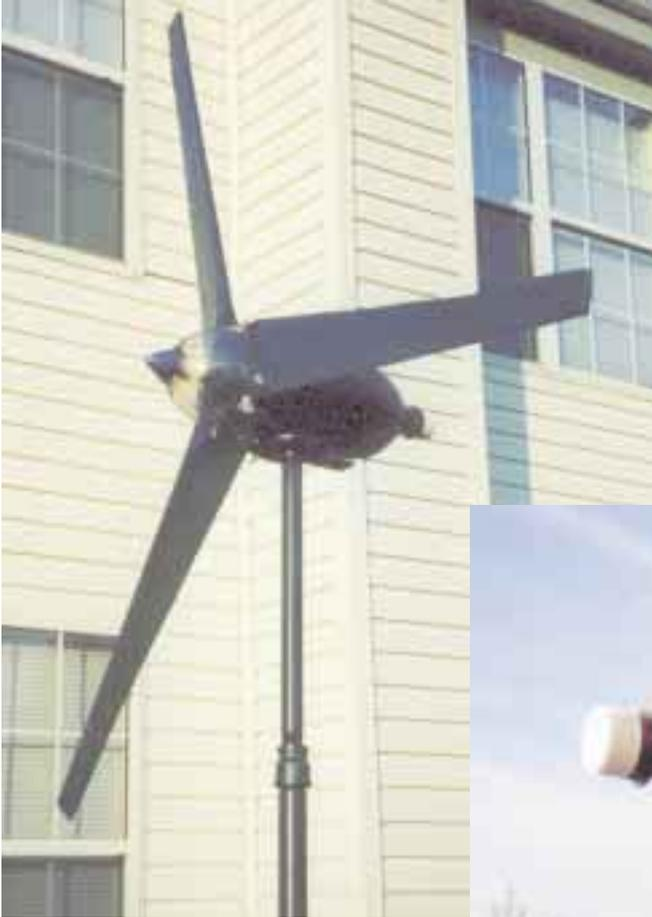
The fixed-mount wind generator with its 3 foot diameter hand-carved wooden blades.
