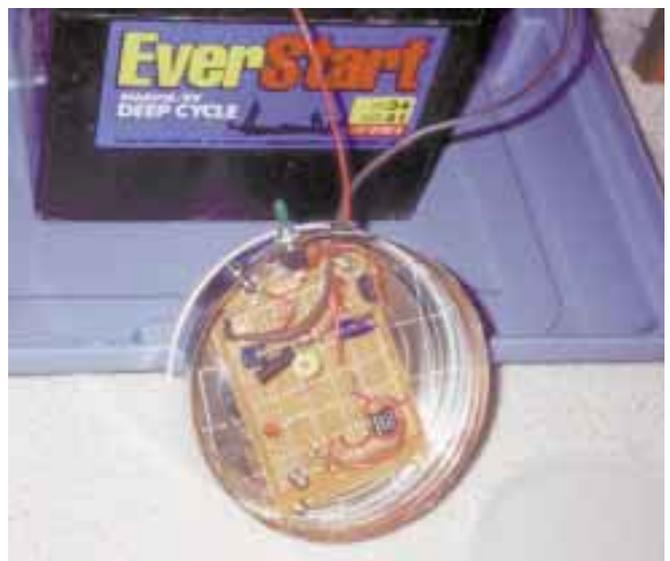
very recent addition and is working to clean the plates of the used cells. Definite improvements were noted on smaller (7 amp-hour) cells after a couple of weeks of treatment; larger batteries take longer. Mr. Cooper has established a BBS on the Web to support the growing interest in this project.
