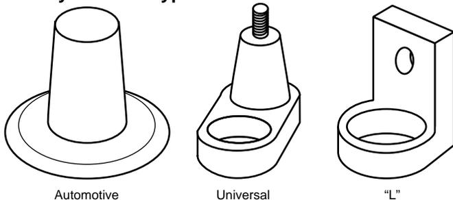
which type of terminal you want on the battery. There are three types of terminals available for the golf cart batteries we use: the automotive terminal, the universal terminal, and the "L" terminal.
