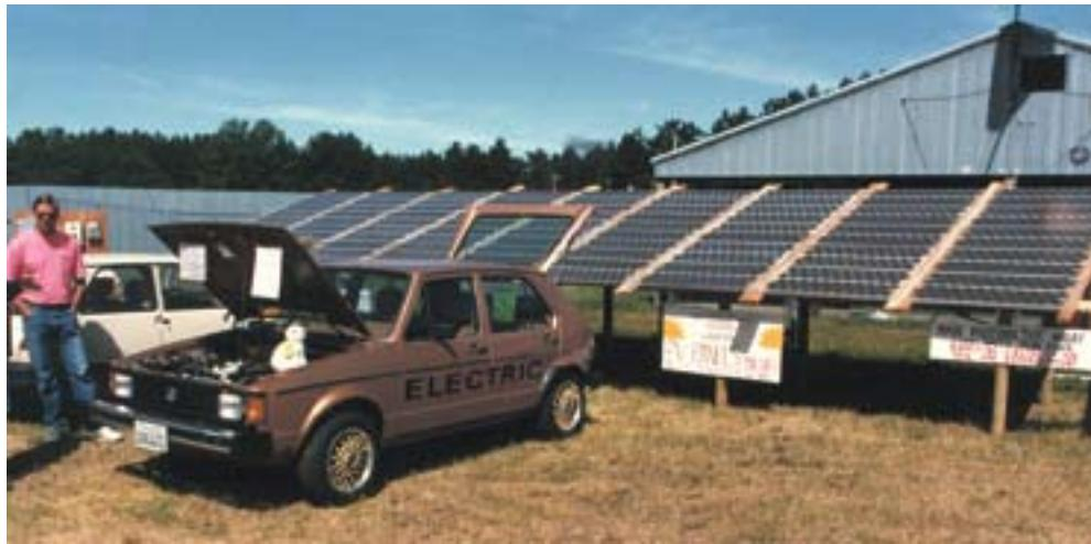
An electric "Voltsrabbit" in front of the 3 KW solar-electric array needed to provide it with a 25-mile average daily range.
