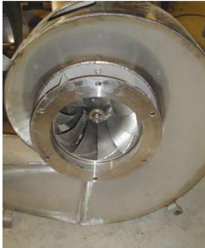
**A Power Pal turbine with a Francis runner direct-coupled to the alternator above.**
