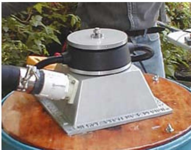
**A Canadian-made Energy Systems and Design turbine uses a permanent magnet alternator and a турго runner.**
