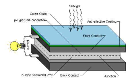
The basic concept here is to convert the sun's rays into an electric current (Shown how above)
