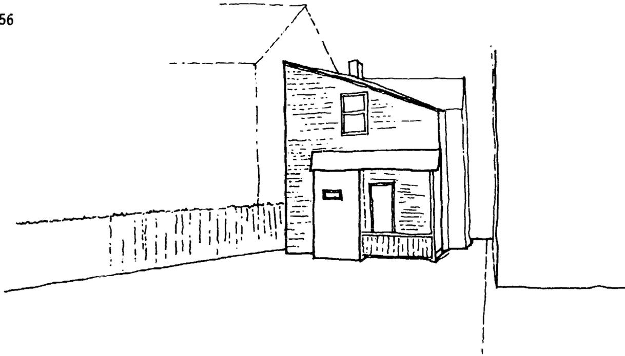
A separate solar collector/heat storage system is used here as the house is blocked from the sun by the higher building to the south. As the house is small, the heat storage must also be outside of it. A window is also added to the western side, as there is valuable heat there too.
