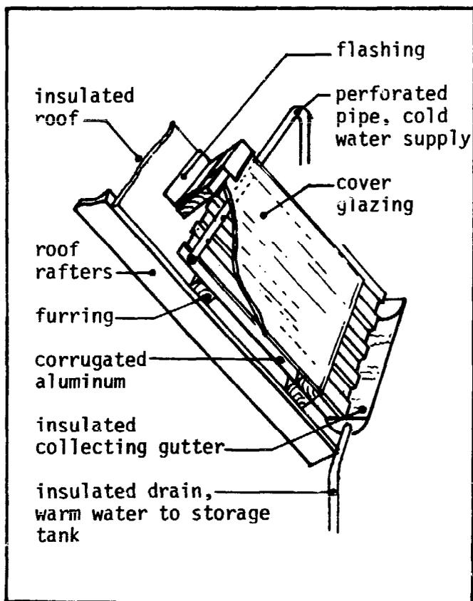
A 1/2 - 3/4 INCH DIAMETER PIPE IS USED TO DELIVER THE WATER TO THE PEAK OF THE ROOF. IT IS PERFORATED WITH TINY HOLES WHICH SQUIRT WATER DOWN EACH OF THE TROUGHS IN THE CORRUGATED METAL. A PUMP MOVES THE WATER UP FROM THE STORAGE TANK.
