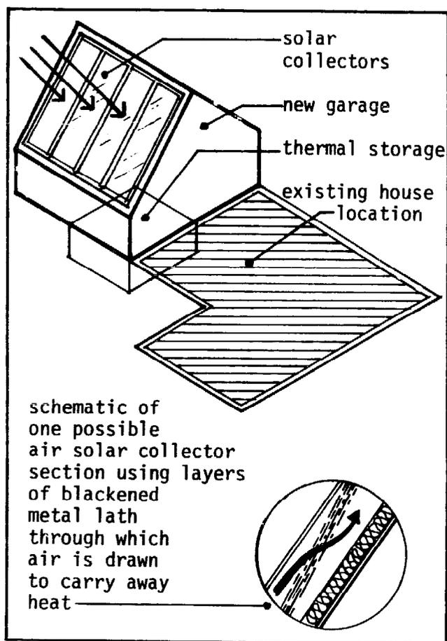
IF YOU WILL BE USING AN AIR SOLAR COLLECTOR YOU WILL BE STORING YOUR HEAT IN A ROCK BIN. THIS BIN SHOULD CONTAIN ROCKS, OF UNIFORM SIZE, WITH DIAMETERS OF 1 1/2 - 2 1/2 INCHES.
