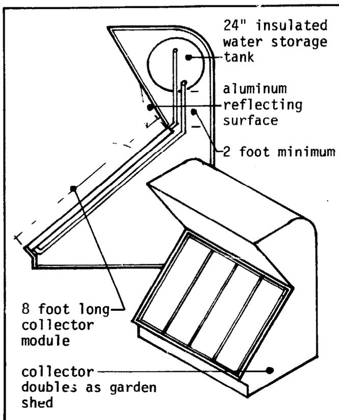
YOUR WATER COLLECTOR CAN BE MADE IN 8-FOOT LONG SECTIONS OUT OF STANDARD DIMENSION BUILDING MATERIAL.
