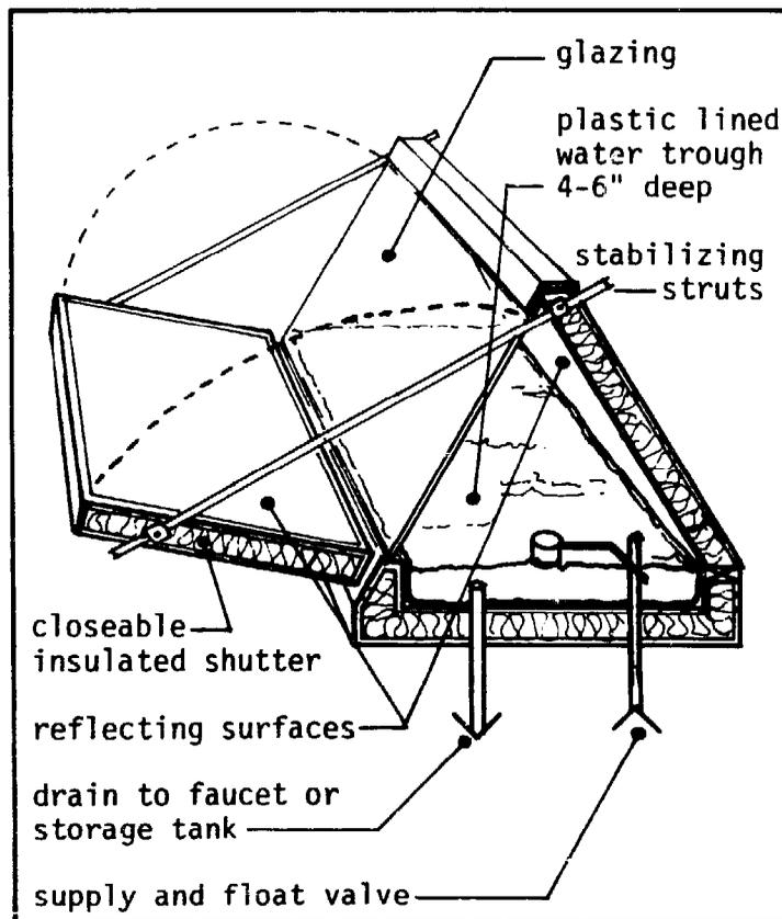
THIS DESIGN CAN STORE HEATED WATER FOR SEVERAL HOURS. THE FILLING AND DRAINING OPERATIONS ARE STRAIGHTFORWARD. OPEN THE SUPPLY VALVE TO FILL IT IN THE MORNING. OPEN THE DRAIN VALVE TO EMPTY IT.
