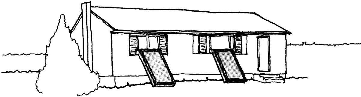
In the simplest improvement, these window boxes increase the solar collection area of these windows. The more complex scheme combines greenhouse frames around each window and a new entry foyer, and solar domestic hot water structure.
