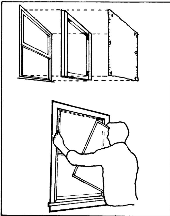
THESE SECOND AND THIRD LAYERS OF TRANSPARENT MATERIALS CAN BE EASILY MADE BY STRETCHING PLASTIC OVER A LIGHT FRAME.
