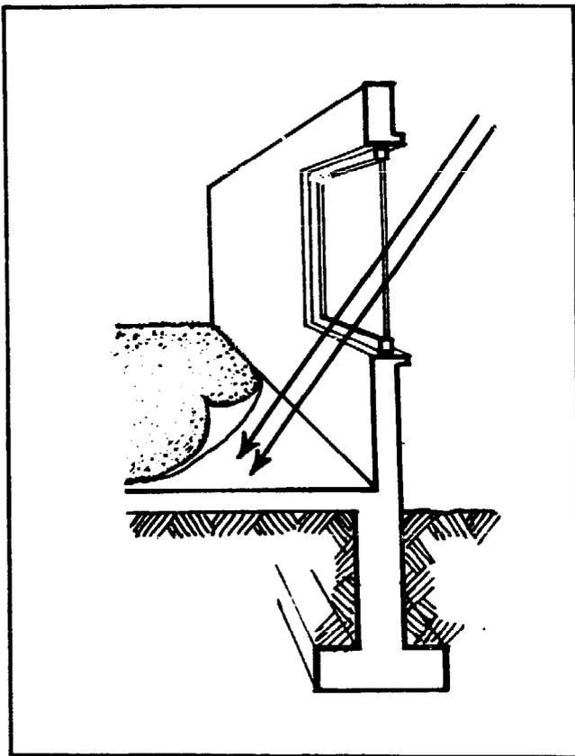
THERE ARE MANY WAYS TO PROVIDE THERMAL MASS TO A ROOM. THE TRICK IS TO GET ENOUGH. TRY TO PROVIDE 2 - 4 GALLONS (1/4 - 1/2 CUBIC FEET) OF WATER PER SQUARE FOOT OF SOUTH WINDOW, OR 1/2 - 1 CUBIC FOOT (75 - 150 LBS) OF CONCRETE OR MASONRY PER SQUARE FOOT. IF THE MASS IS OUT OF THE SUN, DOUBLE OR TRIPLE THESE AMOUNTS.
