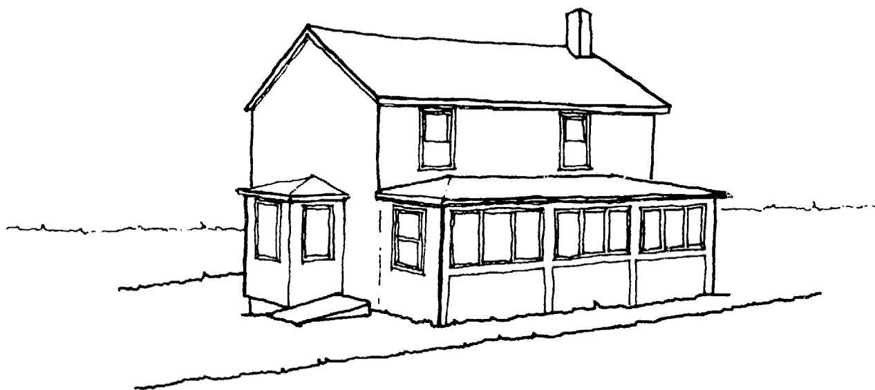
This house is off to a good start as it already has a large glassed-in porch. Outside mounted insulating shutters, with reflective foil faces, would be used to increase the daily input into the porch and then at night be closed to hold that heat in. The slope of the porch roof could also be an effective reflector for a wall-mounted solar collector. Also added is a domestic hot water collector, and more windows.
