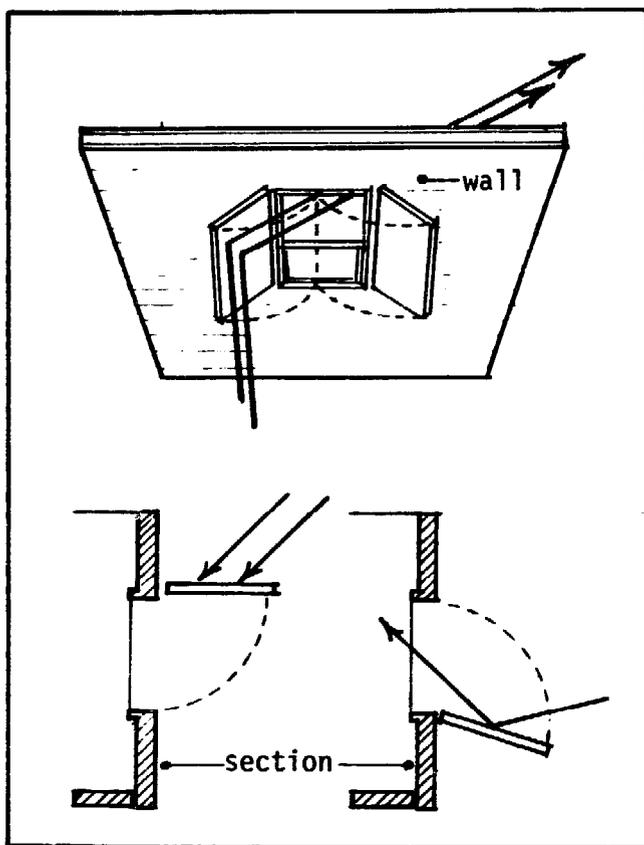
SHUTTER SHOULD FIT SNUGLY WHEN IT IS CLOSED TO HAVE MAXIMUM INSULATING VALUE.
