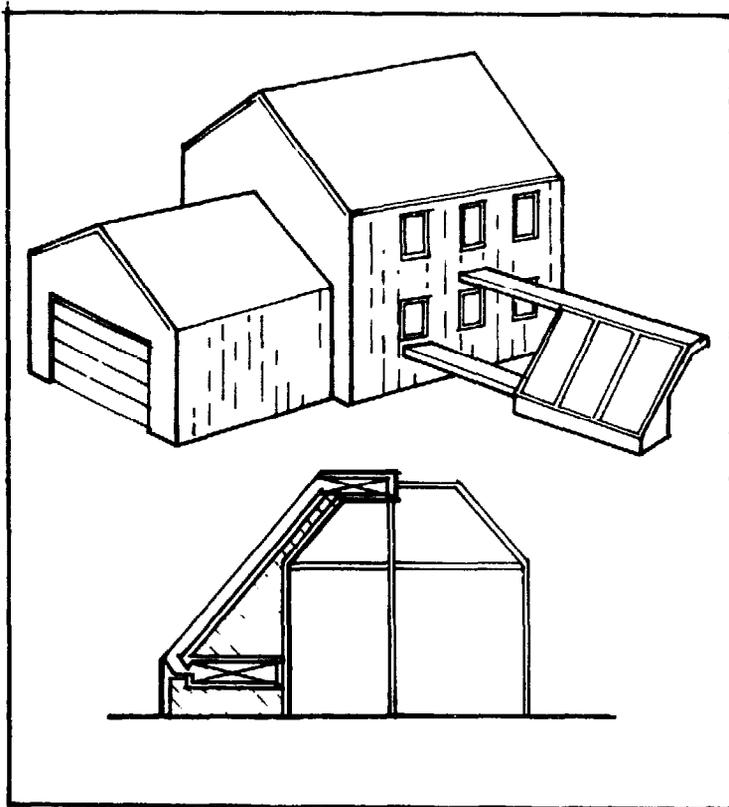
IN SOME CASES IT MIGHT BE POSSIBLE TO ALLOW THE AIR TO RISE NATURALLY THROUGH YOUR COLLECTOR AND BACK TO YOUR HOUSE. IN MOST CASES, HOWEVER, IT WILL BE NECESSARY TO PROVIDE A FAN TO BLOW THE AIR.
