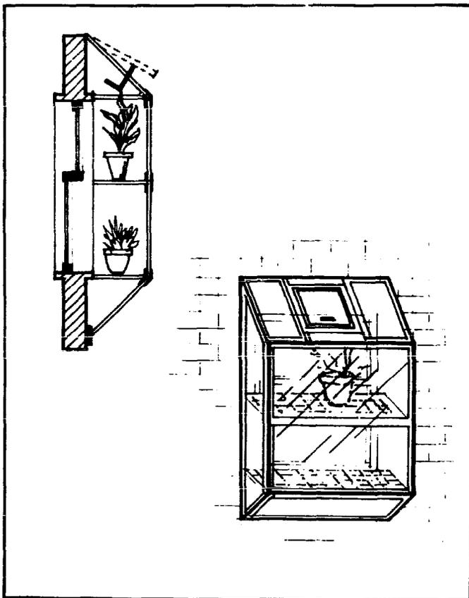
THE FRAME CAN BE MADE OF SOFT WOOD COATED WITH PRESERVATIVE AND COVERED WITH GLASS.
