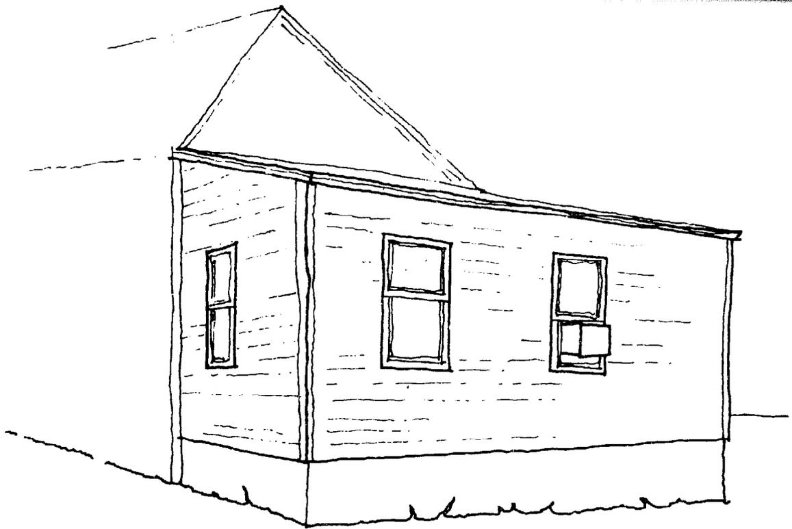
The window box idea here becomes a very large double window box joining two windows. The outside mounted insulating shutters can be used to reflect sunlight into the western facing windows. Both ideas effectively increase the amount of solar energy that enters each window. In the summer the window box could be taken off to keep the heat out and to allow other devices for summer cooling.
