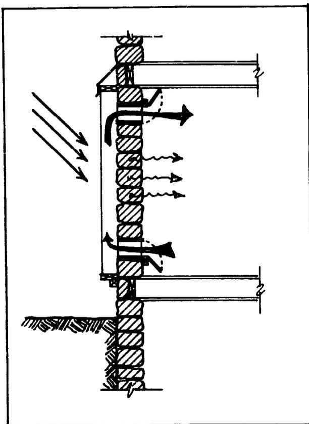
MAKE OPENINGS, FLOOR AND CEILING, EVERY 2 OR 3 FEET. EACH SHOULD BE AROUND 8 INCHES IN DIAMETER. THEY ALSO CAN BE RECTANGULAR.
