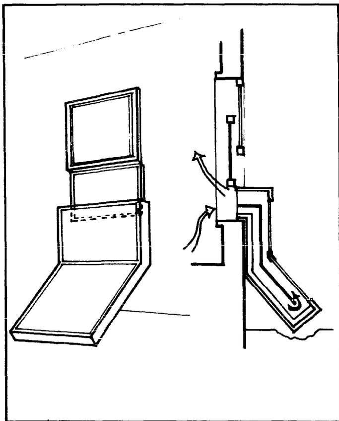
YOUR EXISTING WINDOW REMAINS ENTIRELY IN PLACE. THE LOWER SASH OF YOUR WINDOW ACTS AS A DAMPER; WHEN IT IS UP, HEAT IS ALLOWED IN, AND WHEN IT IS CLOSED, IT PREVENTS HEAT FROM LEAVING THE ROOM.
