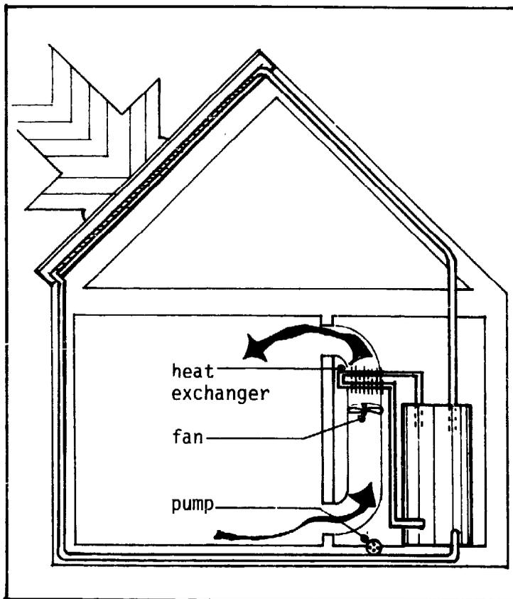
THIS SOLAR SYSTEM REQUIRES A WATER COLLECTOR MOUNTED IN A POSITION FACING THE WINTER SUN. WATER IS PUMPED THROUGH THE COLLECTORS TO A CONVENTIONAL HOT WATER TANK WHICH IS WELL INSULATED (ADD MORE THAN THE UNIT COMES WITH) AND HAS A WATER-TO-AIR HEAT EXCHANGER COIL ATTACHED TO IT. THIS HEAT EXCHANGER CAN BE MADE OUT OF STANDARD 1/2 INCH FINNED COPPER BASEBOARD HEATING PIPES. WHEN HEAT IS NEEDED, AIR FROM THE ROOM IS BLOWN OVER THESE COILS BY A FAN AND OUT INTO THE ROOM AS WARMED AIR.
