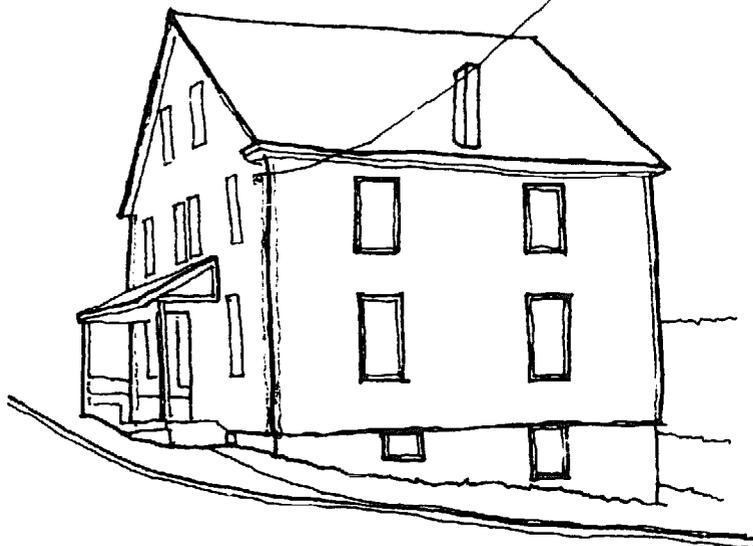
With both yard space and wall space available for solar collection, a lean-to collector/rock storage combination was used entirely across the south face of the building as it did not block the windows. If the building is masonry, it can be partially converted into collectors running vertically up between the windows. The roof angle is good for a pumped domestic hot water heater and the porch could reasonably be enclosed for an entry foyer.
