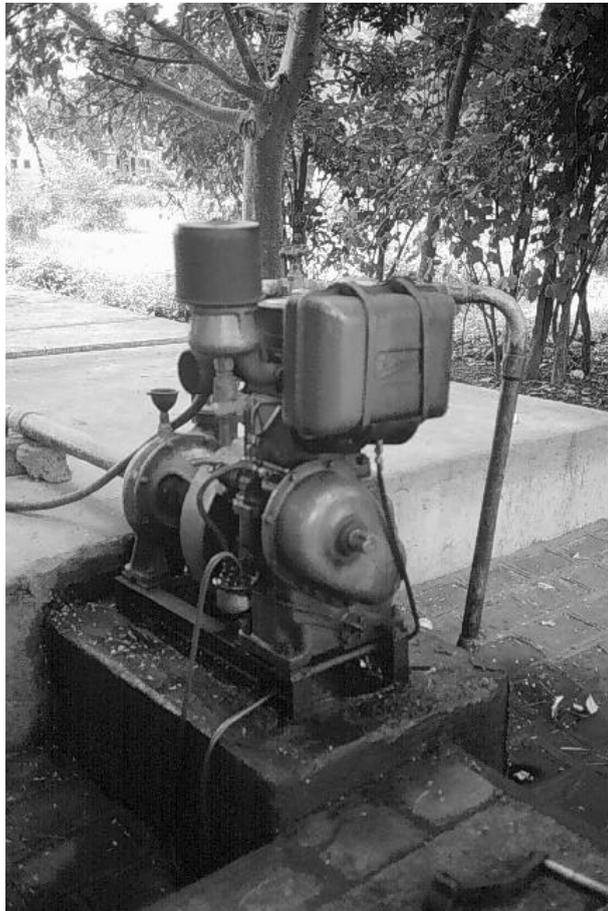
Figure 1: Diesel-driven pump ©ITDG
