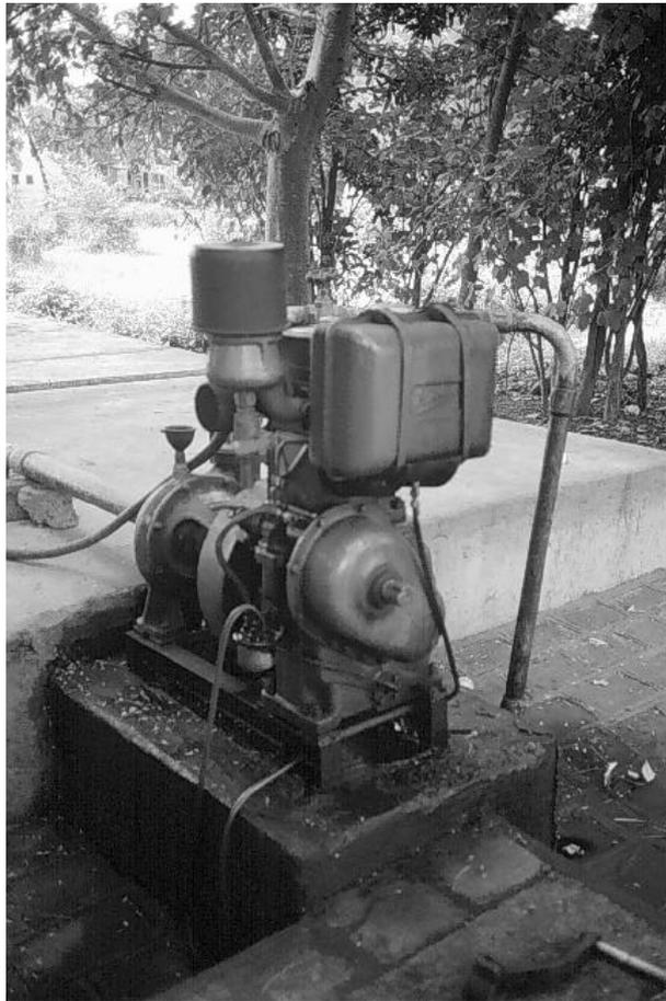
Figure 1: Diesel-driven pump ©ITDG
