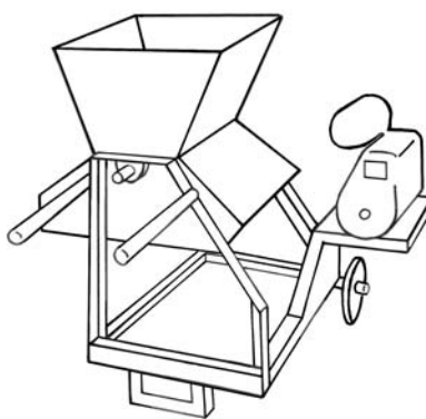
Figure 3: A cassava chipper Illustration: Neil Noble/Practical Action
