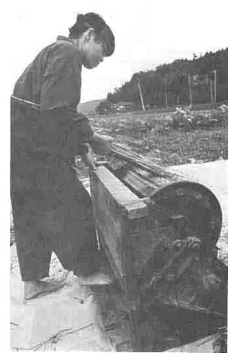
Threshing the crop with the traditional pedal-powered rotating drum (Kyoto). The grains are then winnowed and stored; the straw is returned to the fields.
