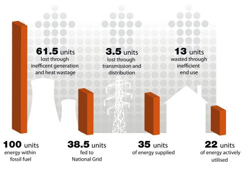
**Figure 1:** Energy losses are inherent in centralised energy systems. *Based on a diagram by Greenpeace*
