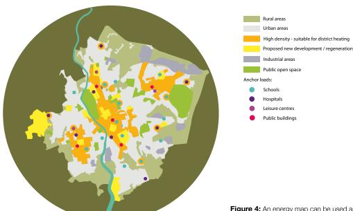
**Figure 4:** An energy map can be used as the starting point for planning and delivering a scheme by project developers
