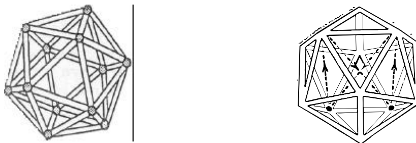
Figure 8: The Icosahedron A: Featuring its Twelve Vertices B: Featuring the Internal Braces
