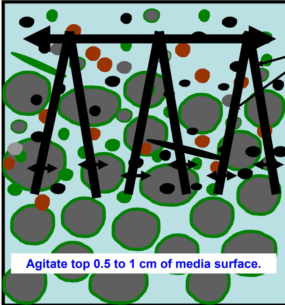
Wire 'fingers', real fingers or a spoon can be used to agitate very top of filtering media where the particles restricting flow are located.
