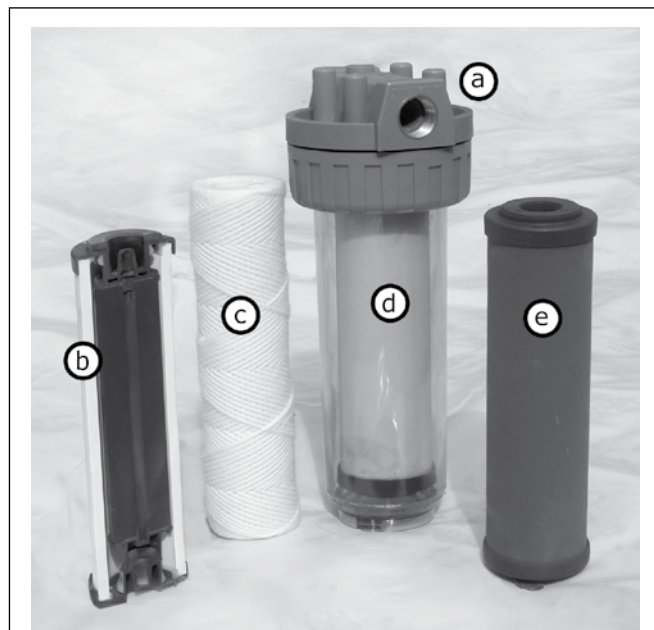
A range of filters are available (a) standard housing unit (b) cutaway version of a combined ceramic and carbon filter: the outer (white) region is ceramic and removes solids whilst the carbon core removes metals, pesticides etc. by adsorption (c) string filter (d) ceramic filter (e) carbon filter.
