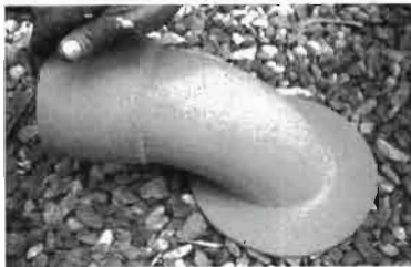
A 4" weld sweep ninety was welded to a flange and painted with galvanizing paint.
