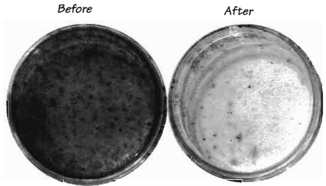
Water before and after sand filtration, after just two and a half days online. As the filter matures, the treatment level will be much higher still.
