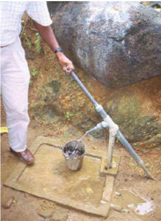
Water is extracted by means of a simple handpump which has been developed, as part of the CWSSP programme, for use with below ground tanks. The pump is known as the Tamana pump, after the Pacific island on which it's predecessor was originally observed (and used for bailing local fishing boats).
