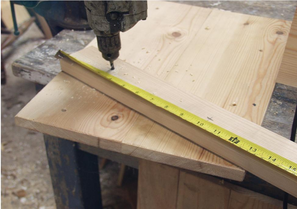
*While you are drilling, you may as well make bolt holes in the legs and end pieces. Mark a point 5" in from the top corner of one of the ends and draw a line to the bottom corner, as shown. The outer edge of the leg will lie on this line. Drill the top hole at least 3" from the top edge, as the tops of the legs will soon be trimmed to accommodate the lid (see below). Ensure that the lower hole falls comfortably outside the line of the side wall.*
