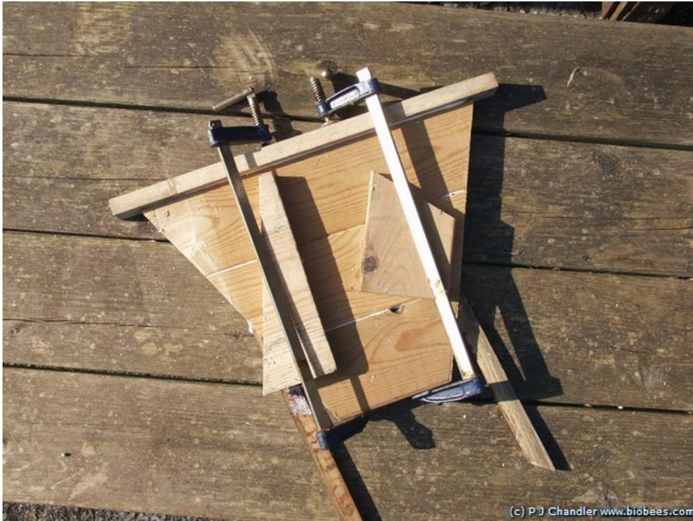
*Glue, pin (or screw) a top bar centred on the top edge of each follower board. Cramp and leave to set overnight. The odd-shaped pieces are there to stabilize the boards while the glue sets.*
