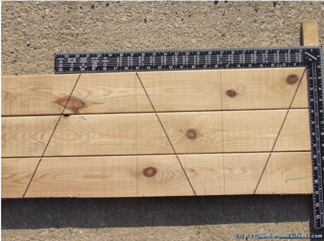
*Extend the geometry to make an identical shape upside down, saving time and timber.*
