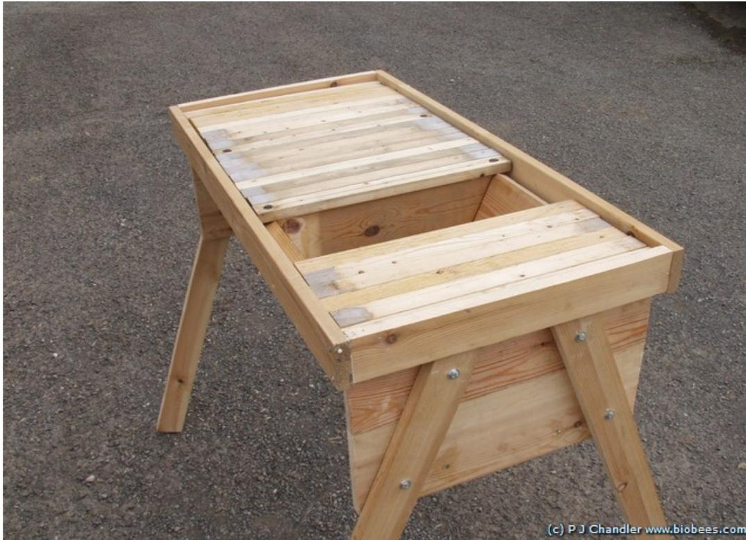
*You can see here how the roof frame is made - a simple, rectangular frame of 3" x 3/4" timber, glued and screwed at the corners. Be sure to leave about 1/4" slack in both directions to allow movement in the wood. Jamming roofs are a nuisance.*
