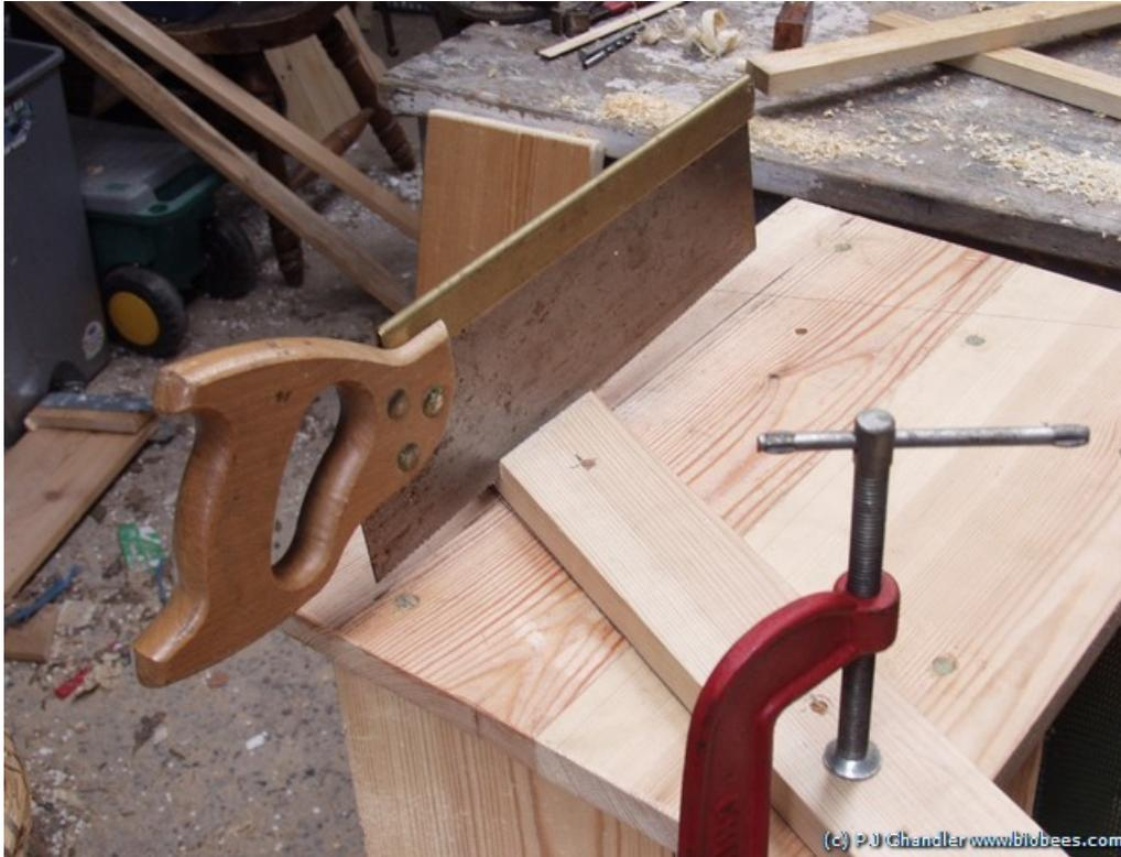
*The roof frame will rest on the tops of the legs, so they need to be trimmed parallel to the top edge. Lining up the holes you already drilled, mark a straight line across the width of one end, 2" from the top edge. Don't fit legs yet.*
