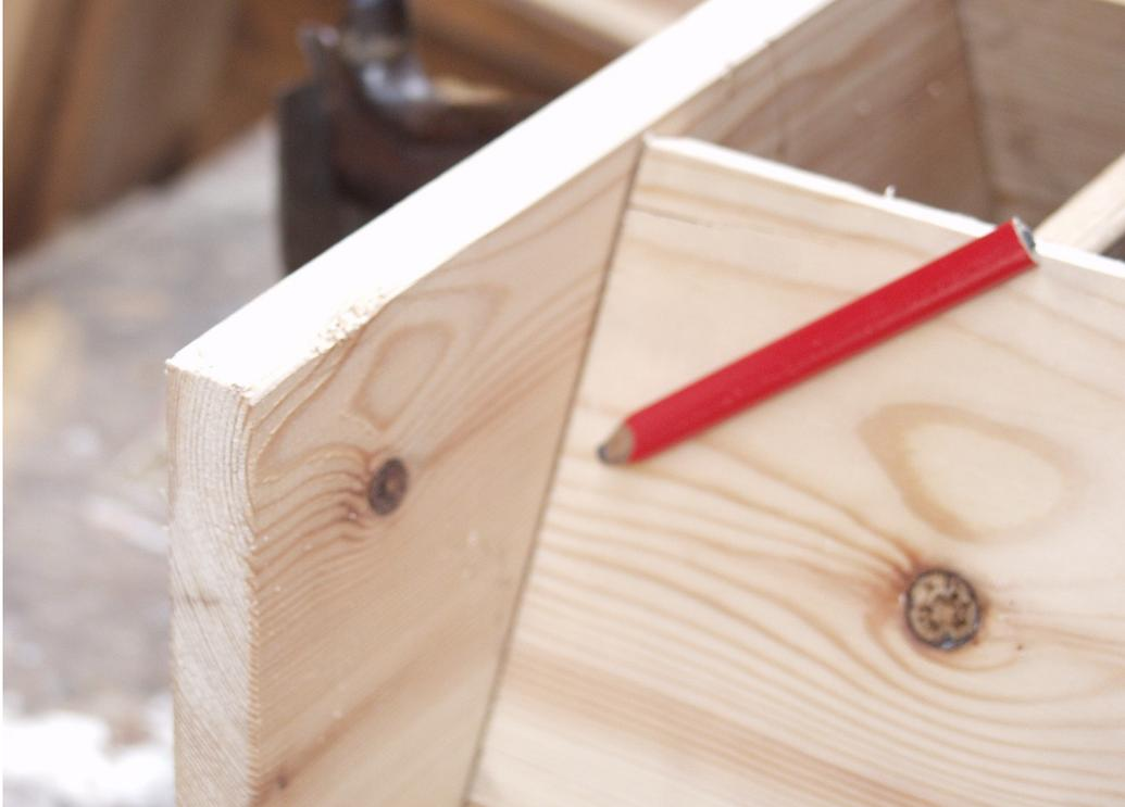
*Make a line where the end touches the sides, inside and out.*
