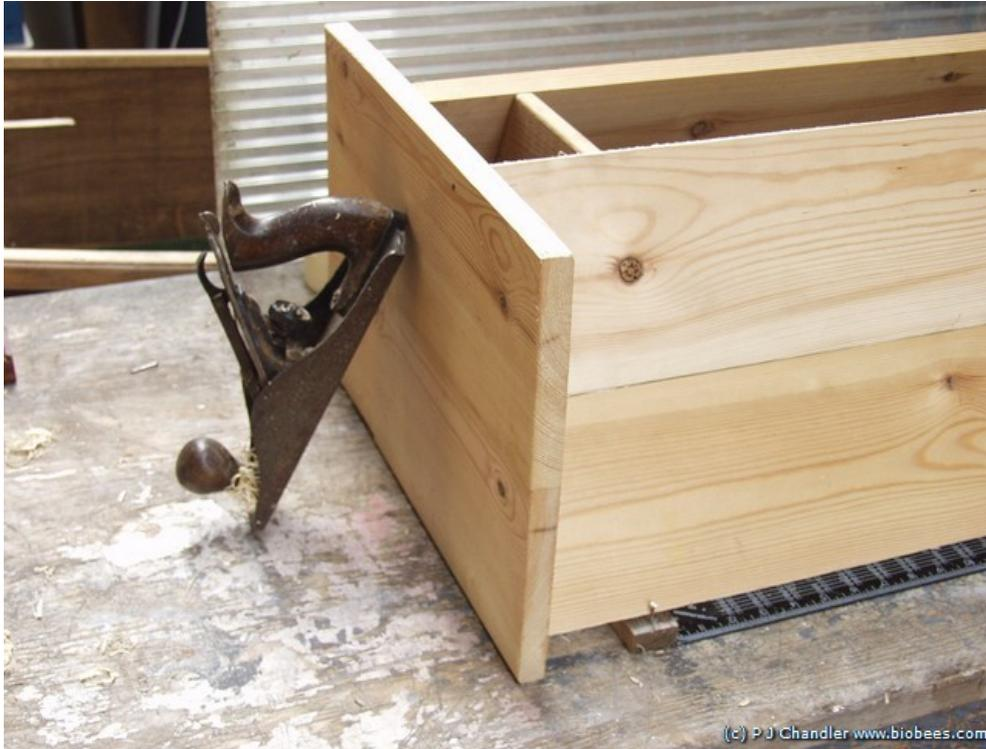
*Position one of the end pieces centrally against one end. Its bottom edge rests on the bench, giving clearance for top bars. (The plane is not necessary - I used it as a prop as I was photographing single-handed)*
