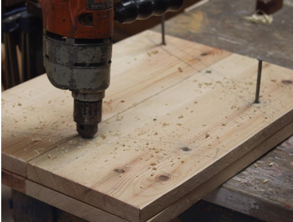
*Use a drill bit slightly bigger than the shank of the screw, which should be brass or stainless steel and at least 2 1/2" long. Drill both ends together, using the marked end as a pattern. (The nails are dropped into two drilled holes to ensure alignment.)*
