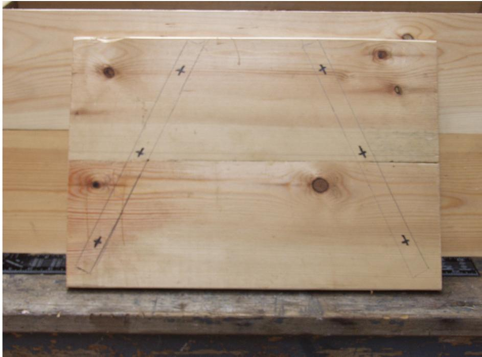
*Remove the end and mark three points each side for drilling clearance holes for screws. Actual positions are not as important as making them on the centre line and away from the ends.*
