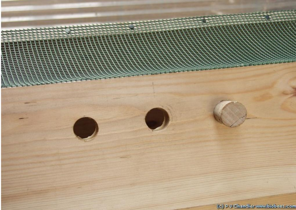
*The bees will need an entrance! Drill three or more 1" (25mm) diameter holes, 2" from the floor, with one in the centre and the other two about 3" either side. Champagne corks or the type (shown here) for closing 1 gal. jars will allow you to regulate the openings.*
