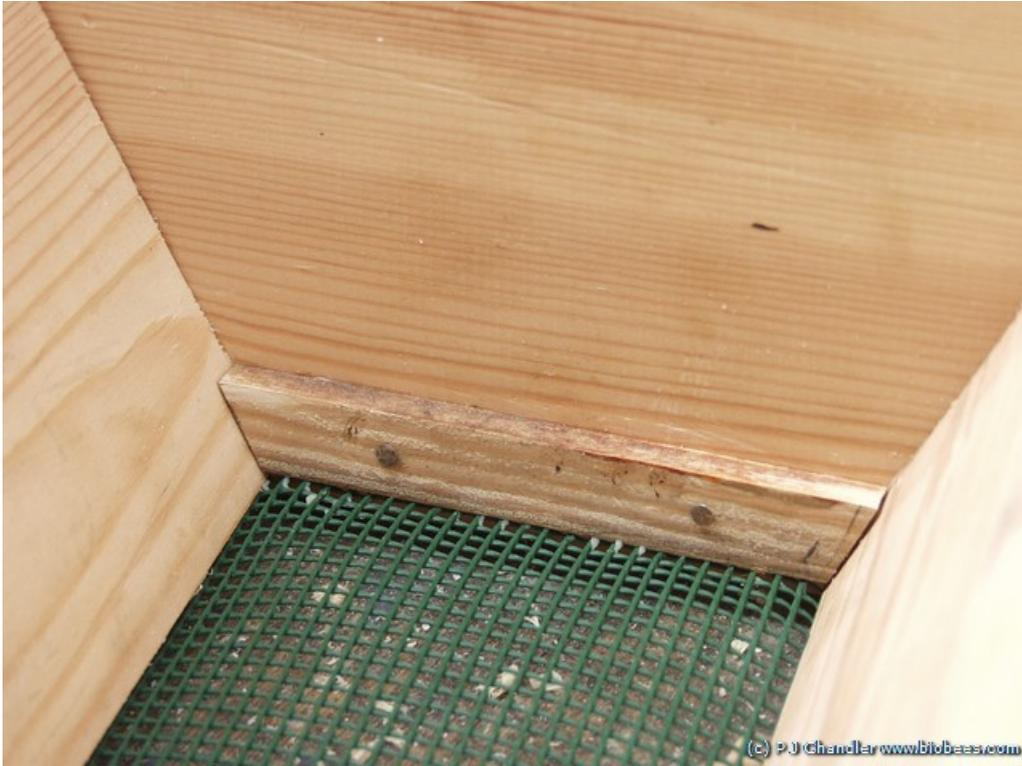
*Glue and pin strips of thin wood inside at the ends, to ensure there are no gaps. Cut them to the shape of the lower ends of the follower boards.*
