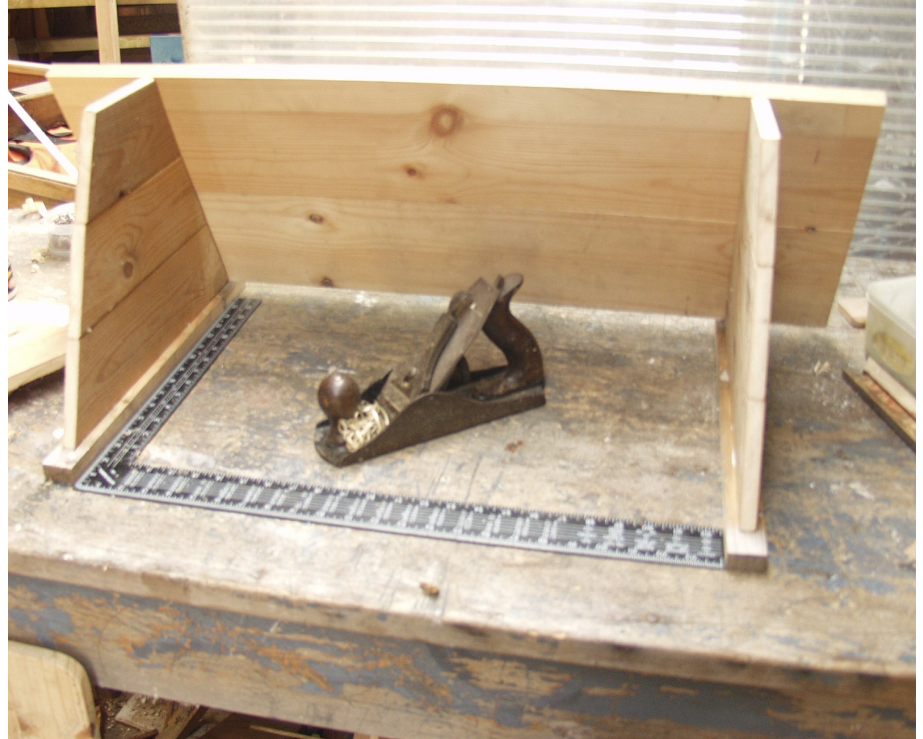
Position one of the side panels against the follower boards, resting on the top bars.
