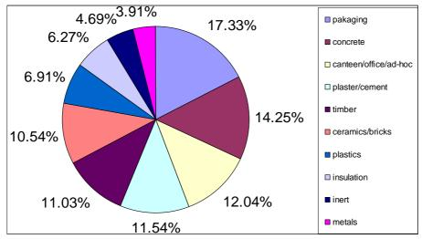
Figure 3 Breakdown composition of construction waste (BRE, 2008)
