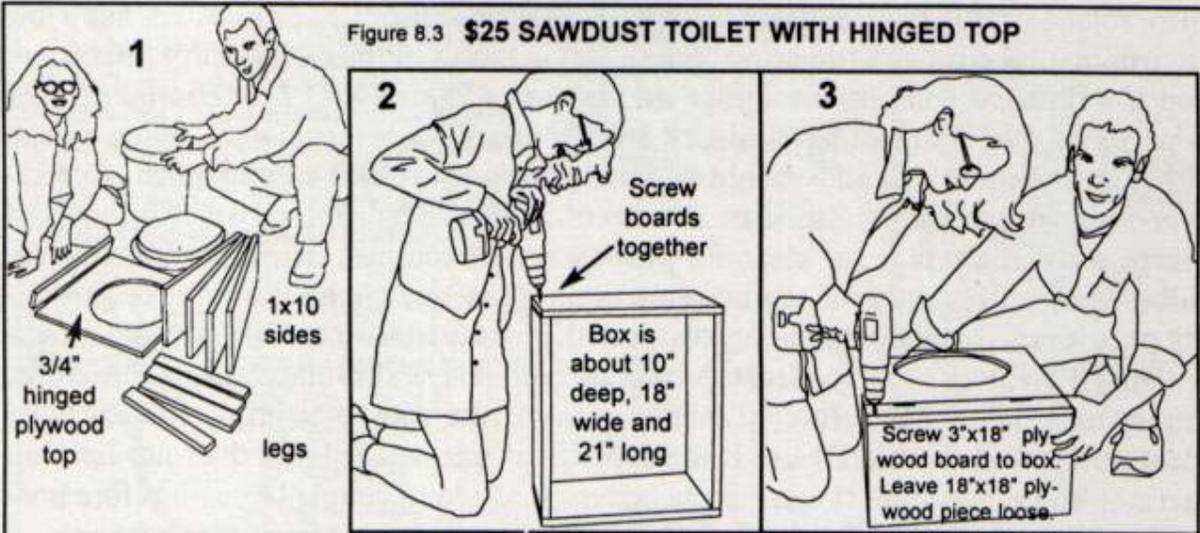
A hinged sawdust toilet box will be 18" wide by 21" long. Get (2) boards 3/4"x10"x18", (2) 3/4"x10"x19.5", (2) hinges, (1) piece of 3/4" plywood 18"x18" and another 18"x3" and hinge them together. Cut a hole in the larger plywood to fit the top of a five-gallon bucket, set back one and one half inches from the front (as in Figure 8.4). Get four five-gallon buckets that are identical. Get (4) 3/4"x3"x12" legs. Get one standard toilet seat.
