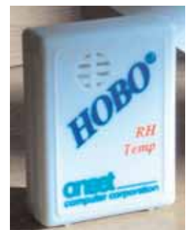
Hobo loggers monitor temperature and humidity
