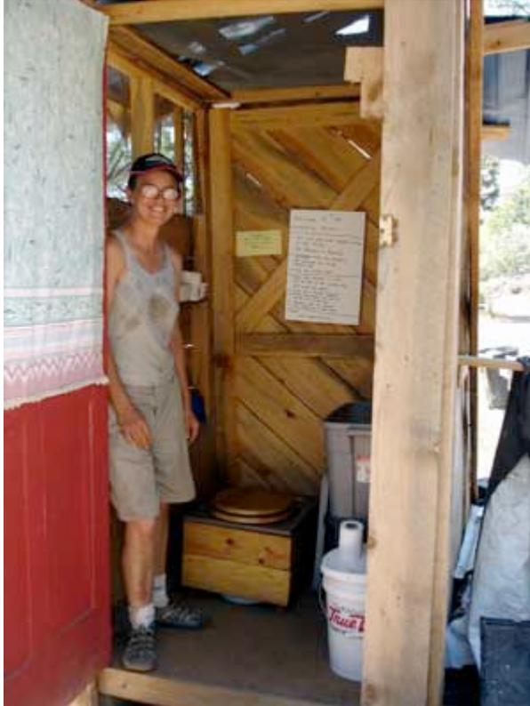
This is the basic toilet (above). There is a white toilet receptacle underneath the seat. The one sitting there on the right is empty, to be used when the one under the toilet is full.
