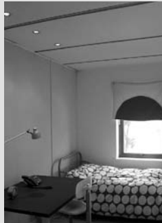
The panels making up the partition wall between the two bedrooms can be moved along the tracks set flush in the ceiling.
