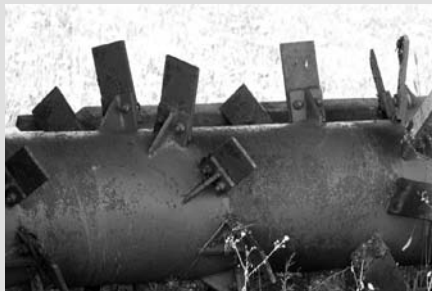
The roller on the compost turner mixes the leaf rows by turning them over.
