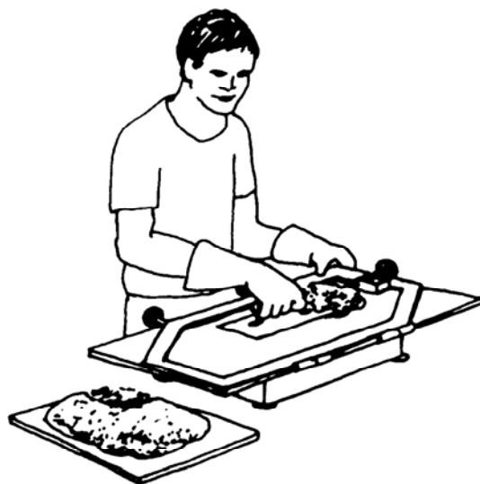
Figure 2: Work the mortar mix under vibration
