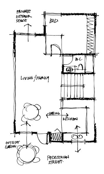
Example of schematic design drawing.
