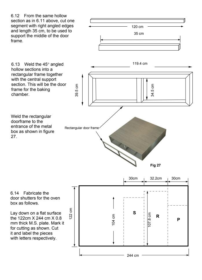
6.15 Cut out segment **R** and divide it into 2 pieces of equal length each of 53.9cm.
