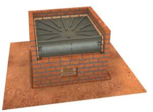
7.2 Cover the top of the oven with the tops fabricated in Fig 41. Place them on the radial hollow segments on top of the oven box assembly They should leave an extension beyond the box of approximately 15 cm on either side across as shown in figure 45.
