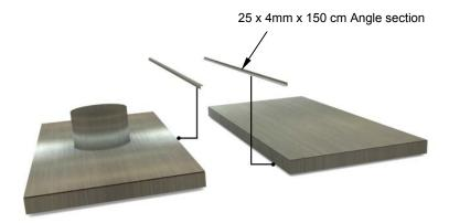
Using arc weld, attach the angle sections to the top covers as shown in figure 32 in order to align the covers and seal the joints to minimise heat escape during the time of oven operation in future.
