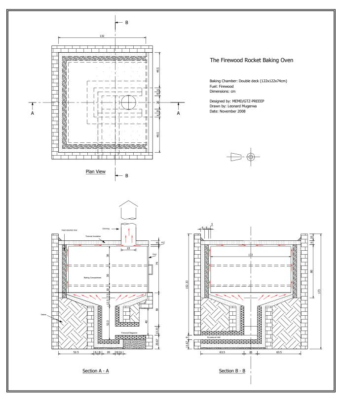
Diagram 9: Technical Drawing of the double deck Rocket Firewood baking oven
