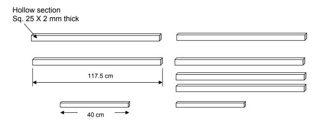
6.6 Cut the ends of the segments at 45°. Select the appropriate segments and assemble them to form an internal support frame of the oven box as illustrated. This will give vertical support in the middle of the oven baking chamber to check sagging when the oven gets hot during baking.
