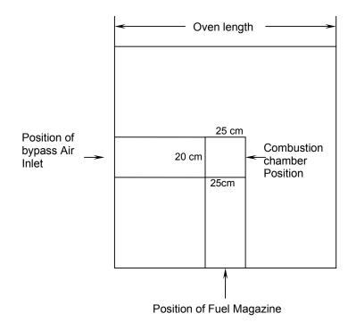
Diagram 3: Positioning the fuel magazine and Bypass air inlet
