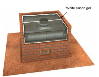
Use silicon gel to seal the joints to minimise possible flue gas leakages between metal joints. This will enhance heat /energy transfer
