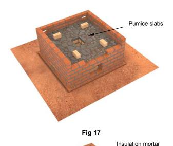
5.18 Lay pumice slabs along the slant to form thermal insulation as shown in figure 17. Use the insulation mortar to bond the pumice slabs.
