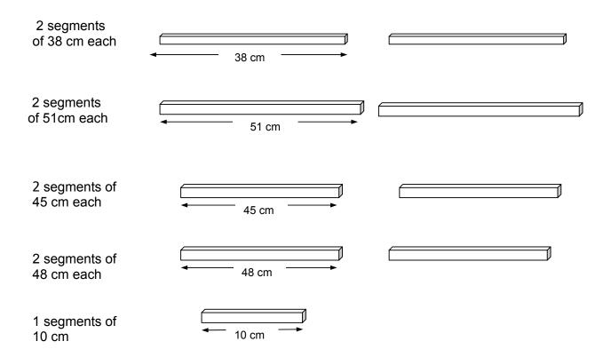
6.23 Position the hollow section segments radially on the top face of the box as shown below. The picture shows the plan (top) view of the box when facing in the direction of the arrow marked F.E. (see Diagram 9). Use arc weld to fix them into position.
