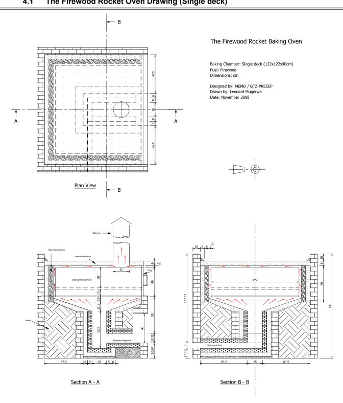
Diagram 2: Technical Drawing of the single deck Rocket Firewood baking oven
