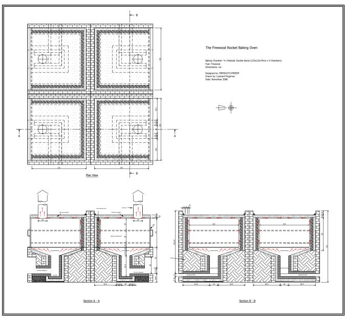
Diagram 10: Technical Drawing of the large scale rocket firewood baking oven
