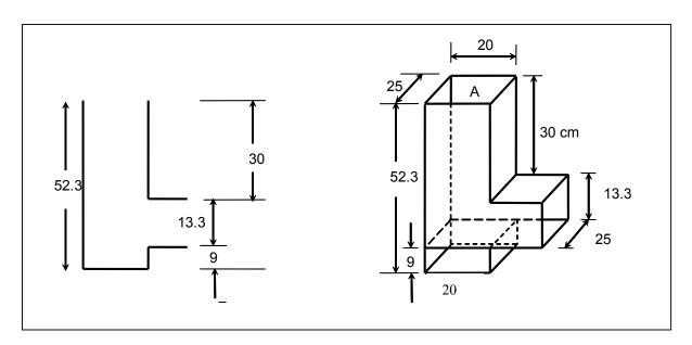
Diagram 4: Details of the combustion chamber size (Dimensions in centimeters).
