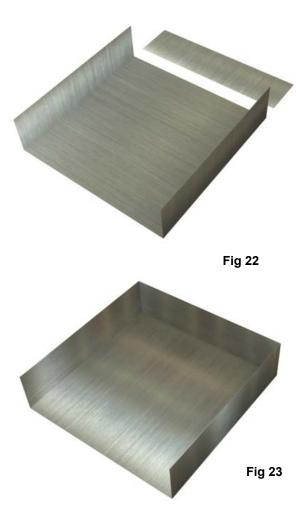
6.4 Lay down on a flat surface the 1220 x 2440 x 2mm MS plate (= 4' X 8' X 2 mm), and then mark it for cutting as shown below.
