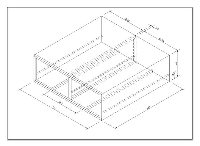
Diagram 5: Illustration of the metal oven box for the single deck oven (120 x 120 x 40cm)
