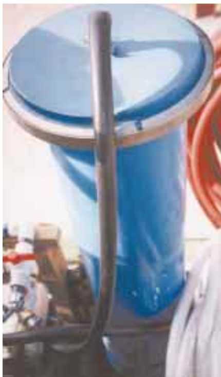
Left: A fuel filter, salvaged from a tug boat, gets the bits of french fries out of the cooking oil.
