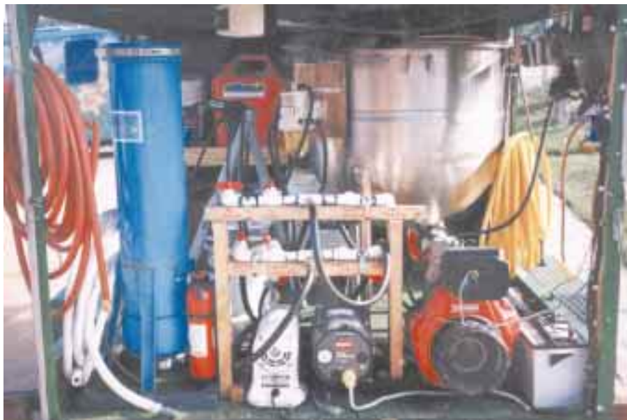
Below: The Green Grease Machine performs transesterification.
