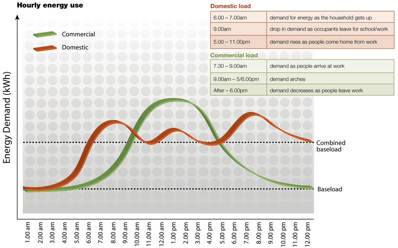
**Figure 6:** This graph shows a typical domestic and a typical commercial load profile, and how they complement each other
