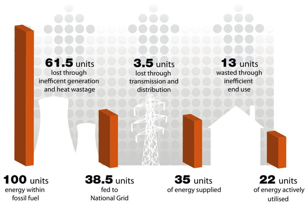
**Figure 1:** Energy losses are inherent in centralised energy systems.
