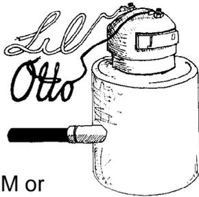
Lil Otto is a permanent magnet hydroelectric generator. He works with as little as 1.2 GPM or Heads as low as 20 feet. 12 or 24 VDC output, up to 5 Amperes. Comes complete with manual and right nozzle for your site.
