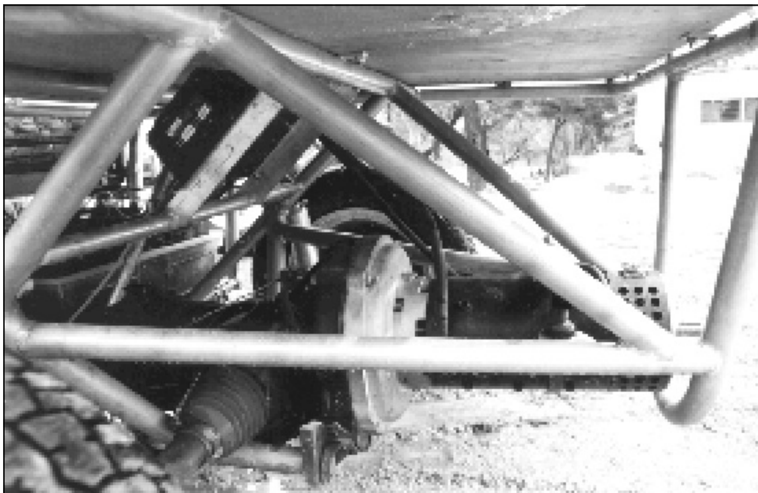
Above: A solar powered electric motor replaces the old dead dinosaur burner.
