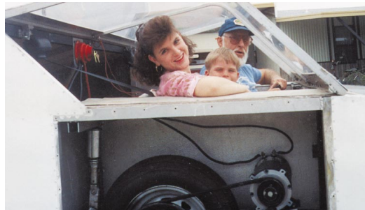
Right: Grandpa (Capt. Burt Newland) gives Monica & Herby Bretch a solar ride. Panel is removed to show motor & wheel assembly.
