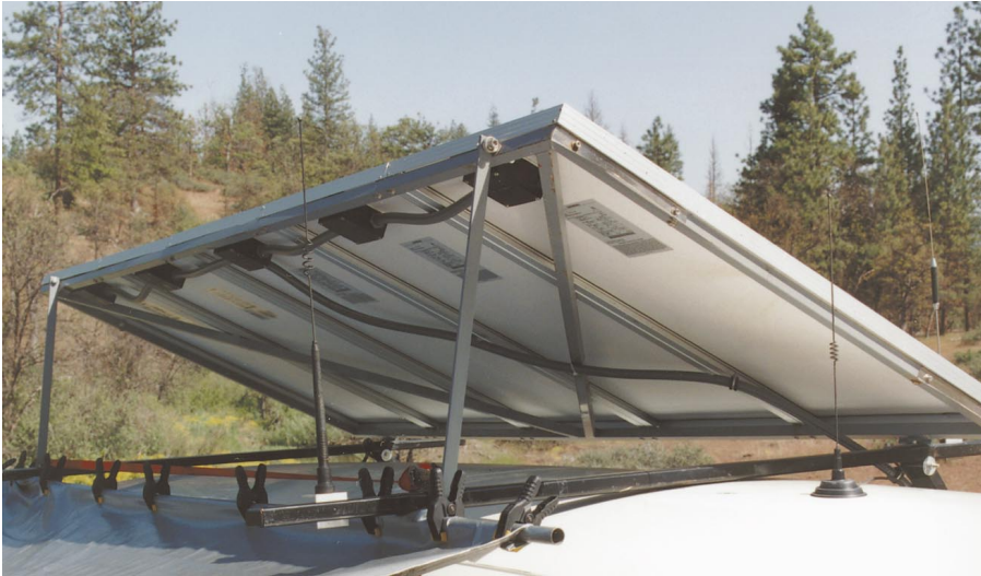
Above: Detail of the custom-welded tilt-up rack and its five Siemens PC4-JF photovoltaic modules. Note the flexible conduit between the modules.
