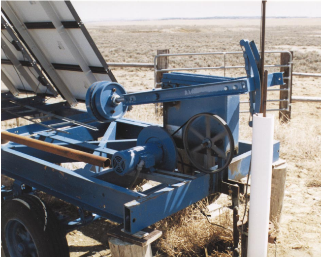
Above: Detail of the jack pump assembly and the 90 Volt DC motor.
