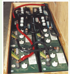
The batts: eight of the sixteen 220 amp hour batteries in Sun Chaser's hold.
