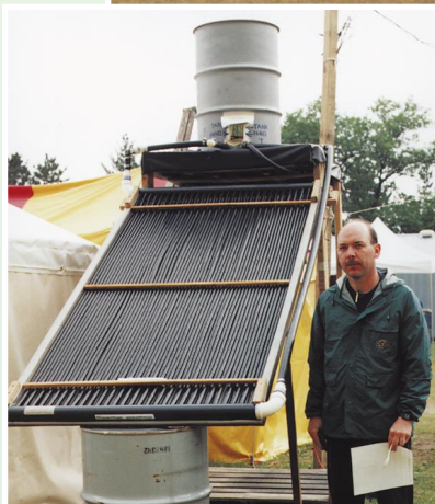
Do it yourself: James Machacek sells plans and custom manifolds so you can build these simple thermosyphon water heaters.
