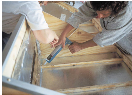
Above: Siliconing the oven.
