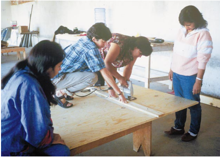
Above: Cutting the wood for the oven frame.
