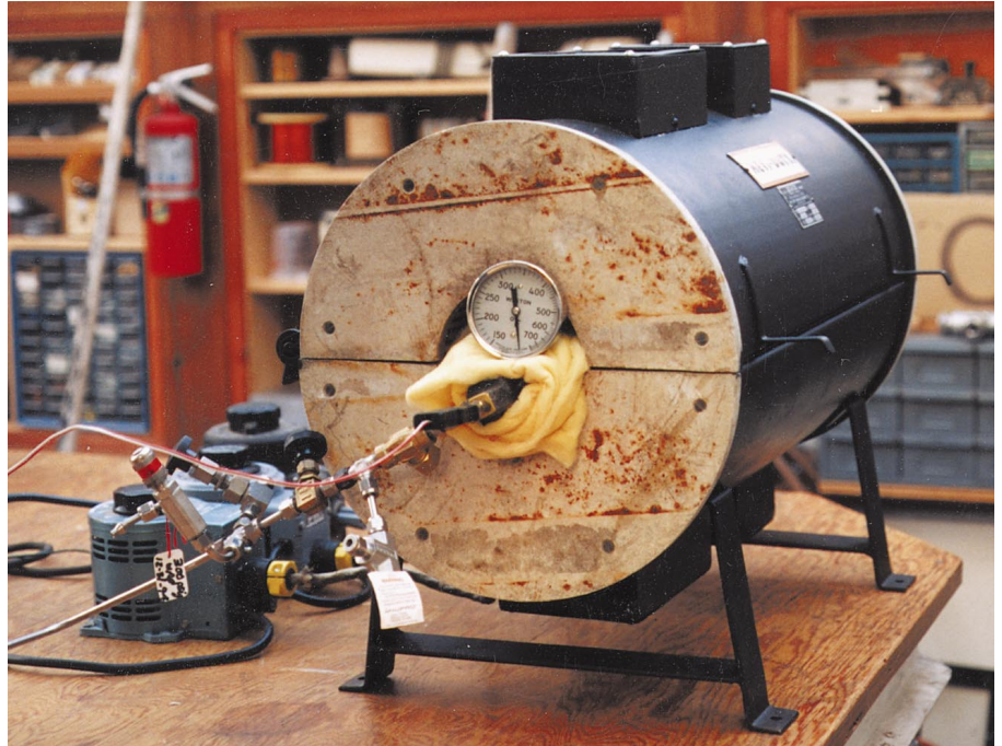
Above: Electric tube furnace ready for activation of MH cylinders.
