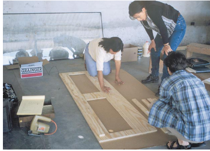
Above: Making templates of the oven so it can be easily replicated.
