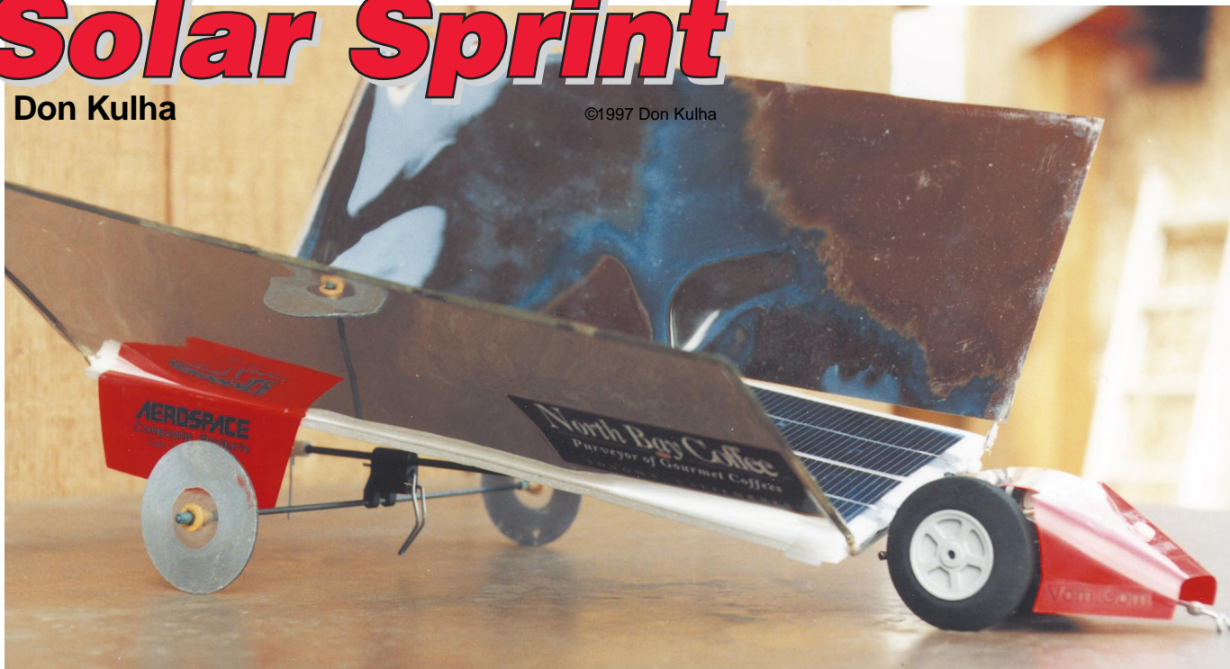
Above: PV panel angle adjustability aids collection of maximum energy.
