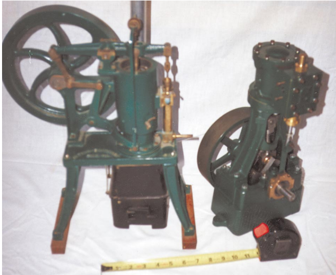
Above: Ryder-Ericsson with pump, 500 gallons per hour to 50 feet.
