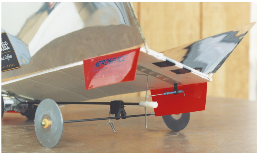
Below: Adjustable mount attaches panel to chassis and allows easy and accurate angle changes. Note line guide below rear axle.
