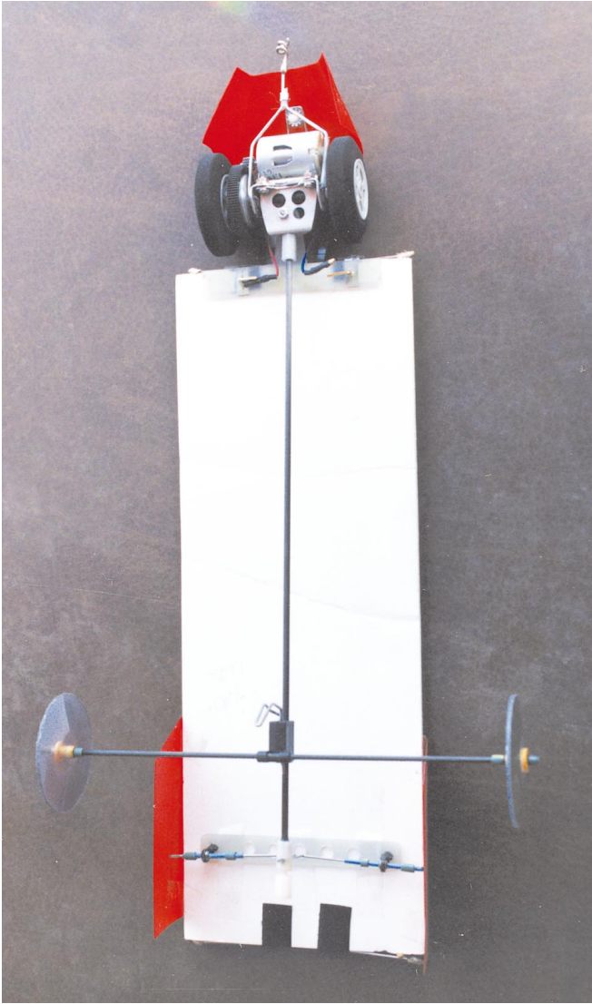
Above: Long wheelbase aids directional stability and aerodynamics with little weight penalty.
