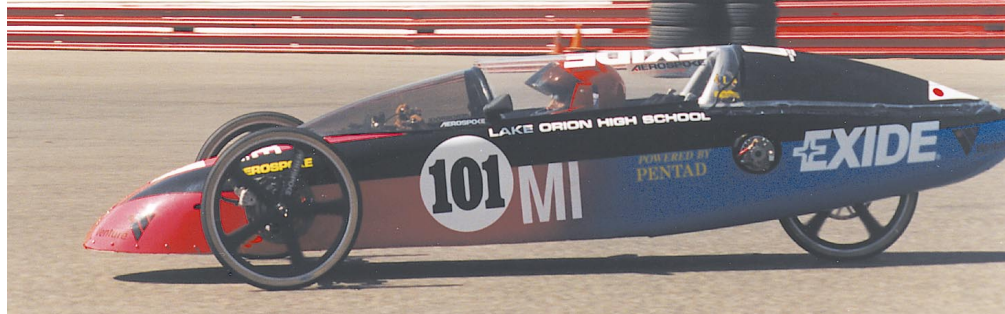
Above: This low sleek shape is typical of Electrathon bodies.
