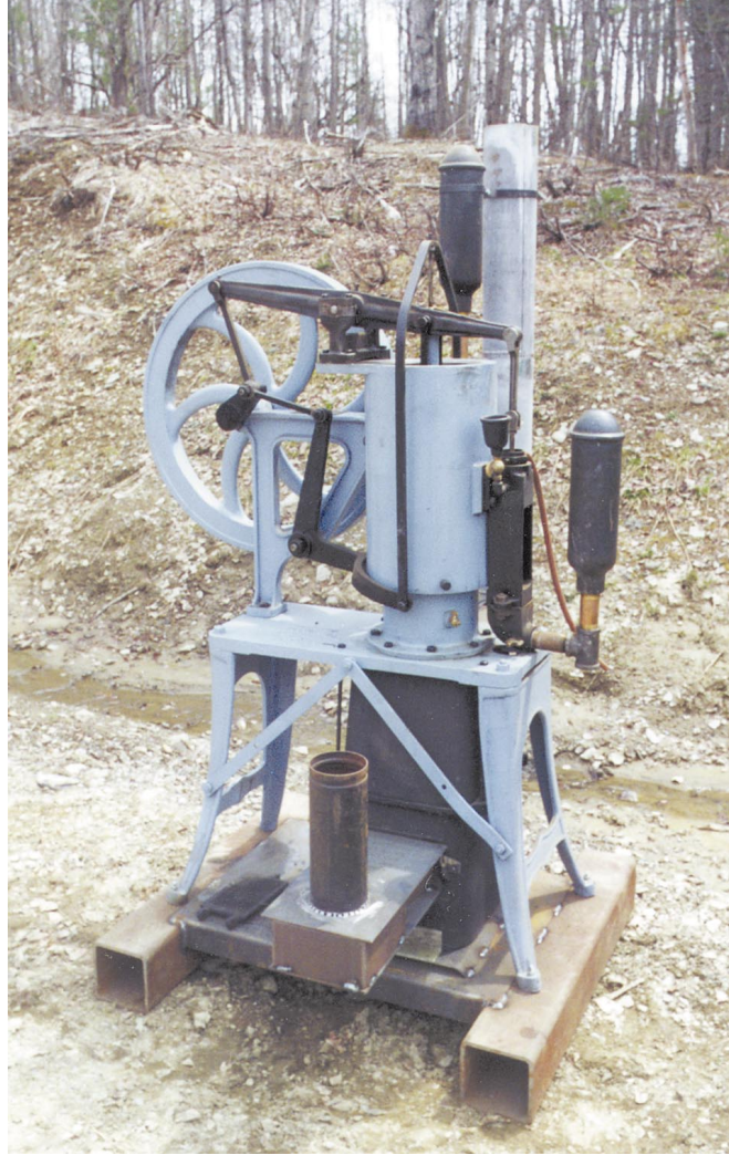
Above: A Civil War era Rider-Ericsson Stirling cycle engine restored by Charles Mac Arthur.
