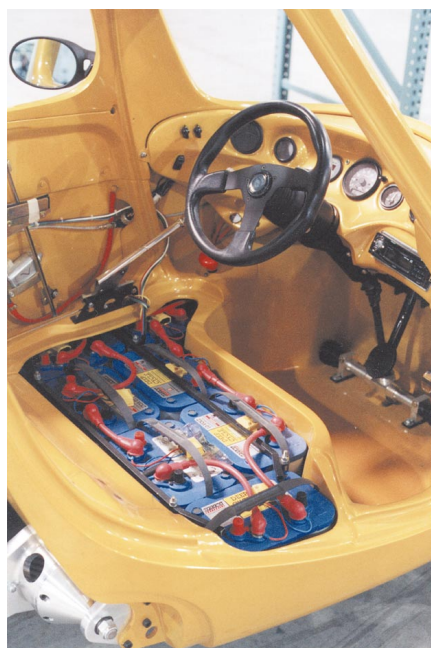
Left: Some of the thirteen sealed lead-acid batteries are stored under the seat.
