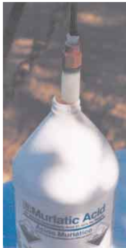
Above: The ozone diffusing stone after cleaning with Muriatic Acid.
