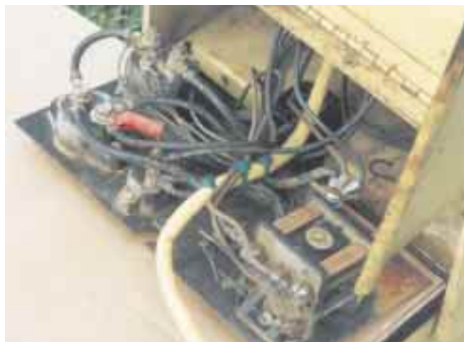
Below: The opened access panel on an E10. The larger relay on the right is the PTO contactor.
