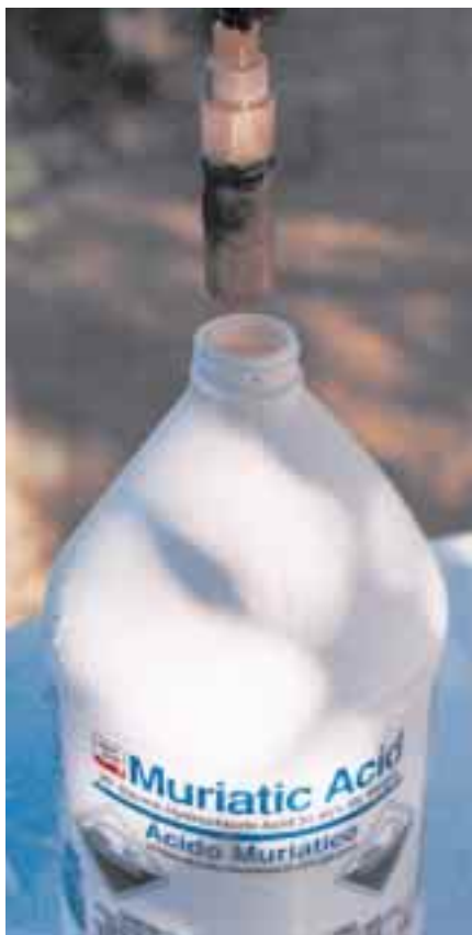
Above: The ozone diffusing stone clogged with impurities.
