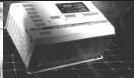
TRACE Sine Wave 4000 Watt Inverter / Charger. 10,000 Watt Surge Power with 2800 Watt Charger. Fully programmable, including control of generator and relay closures. Stackable for double the power.
