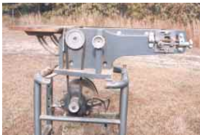
Left: A 12 volt 1/2 hp 1,725 rpm Delco motor found at a flea market powers this belt sander.
