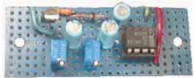
Above: The components laid out on perfboard.
