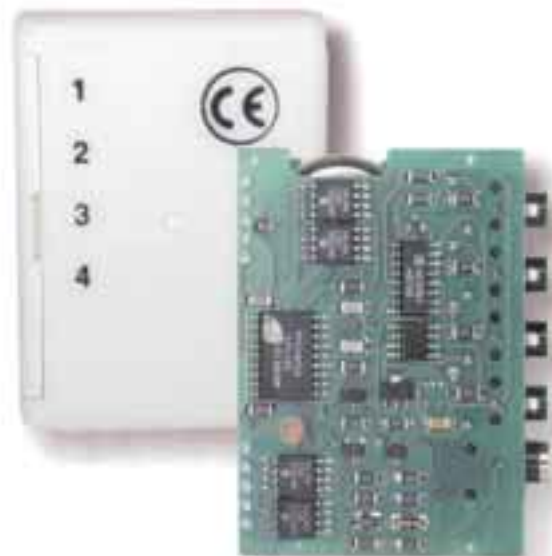
The case and brains of an Onset HOB0 four channel external data logger.
