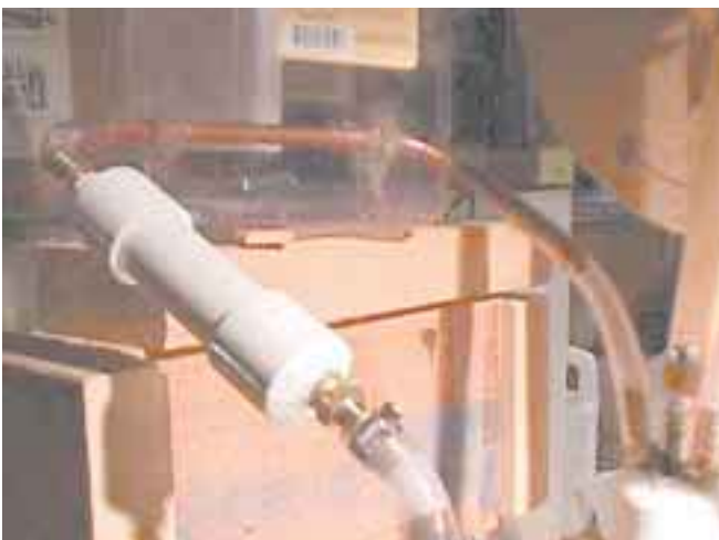
Photo 5: Regenerator and cooler.
