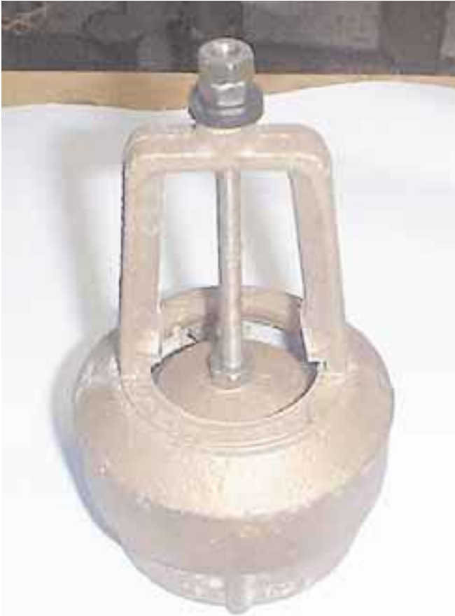
The modified foot valve ready to assemble onto the ram.
