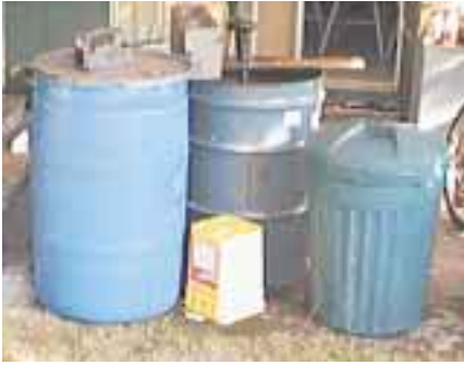
L to R: storage drum, mixing drum, and sodium methoxide mixing drum.
