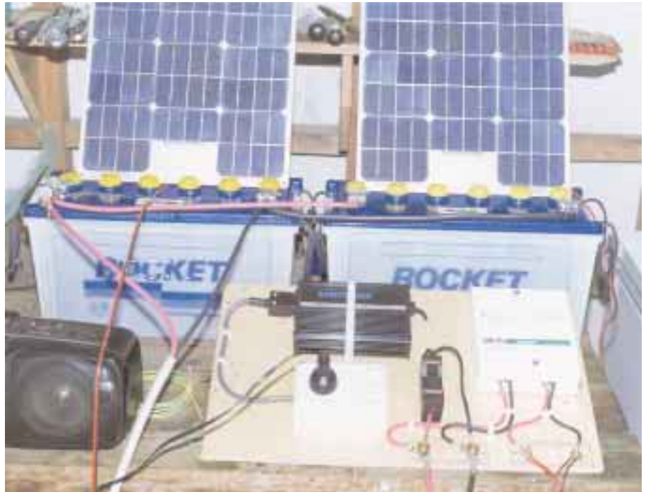
The system as bench tested at Mt. Hagen (the small solar panels were only used to test the charge controller).
