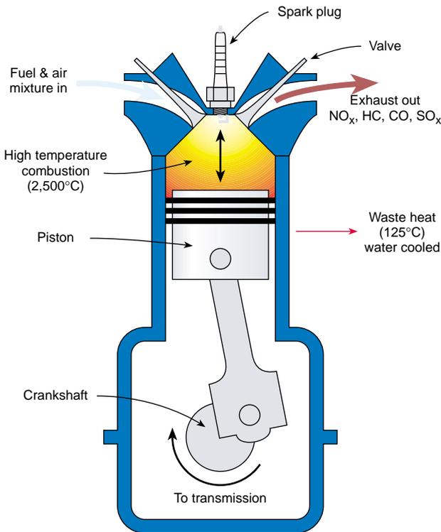
Rotary mechanical output: 20% power efficiency
