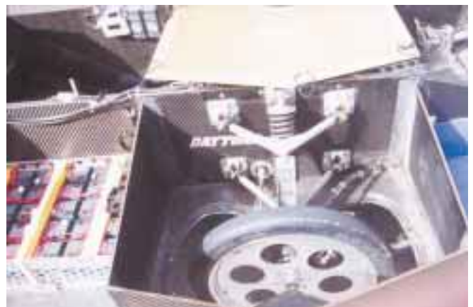
Front suspension, double wish bone, and Dunlop Super Solar tire.
