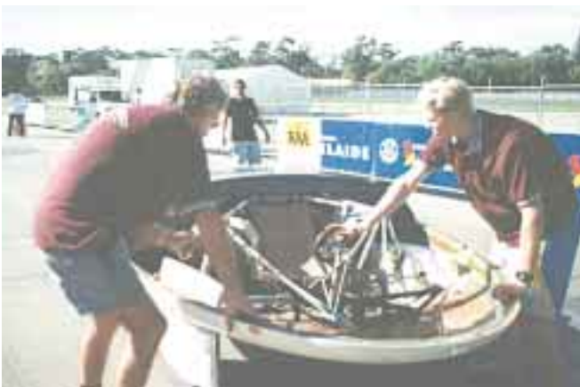
A welded cromolly chassis with a fiberglass shell. One of the heaviest entries, at over 660 pounds (300 kg).
