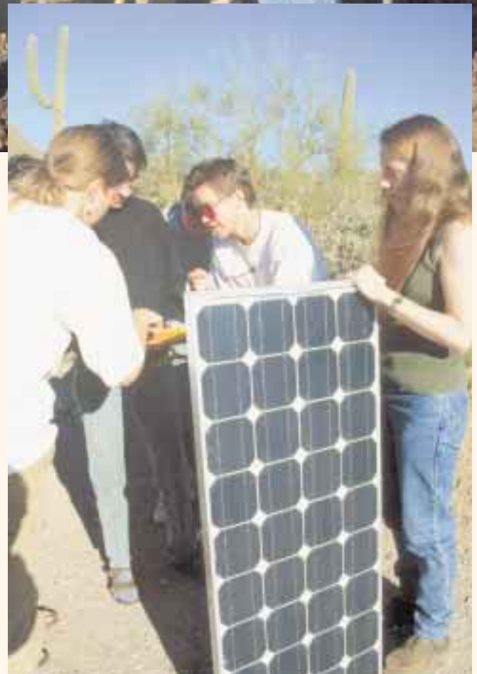
Above: Solar sisters. Right: Testing short circuit current and open circuit voltage on a PV module.
