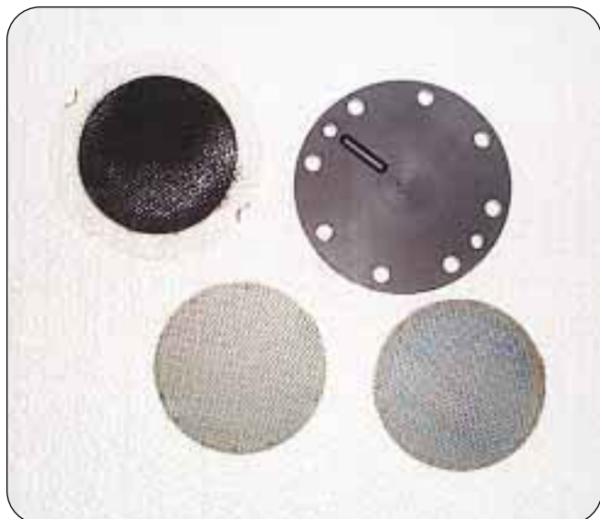
Membrane and nickel electrode screens for the PEM electrolyzer.
