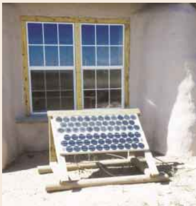
These Arco and Photowatt 50 watt modules are used in the 12 volt, DC-only system.
