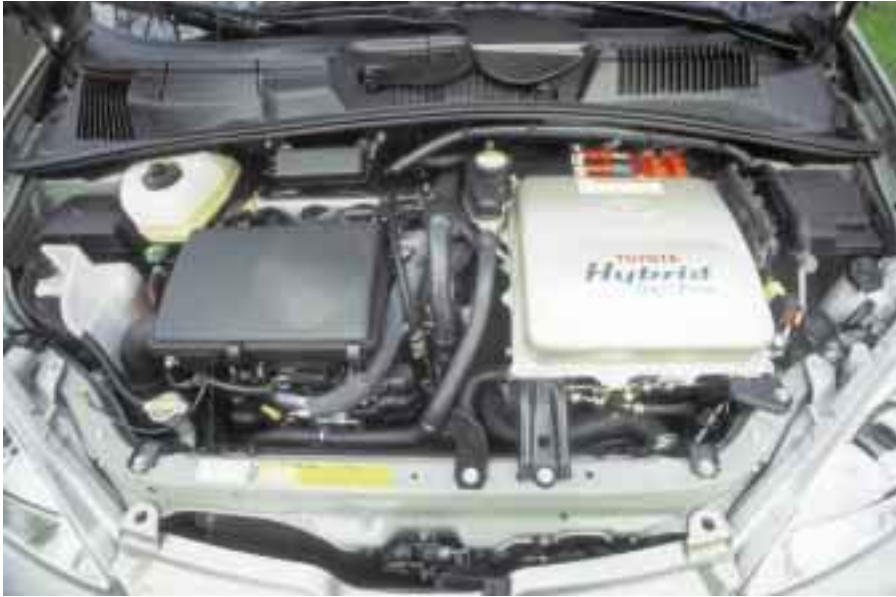
Under the hood—the gasoline engine and electric motor/generator.
