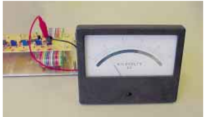
An analog meter may be used in place of the digital display.
