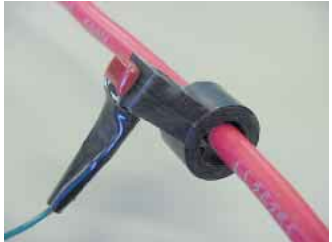
Close-up of the Hall-effect sensor and stabilizer capacitor. A major advantage of the Hall-effect current sensor is its isolation. It may be placed on either the positive or negative line. It is shown here measuring current in a positive line.
