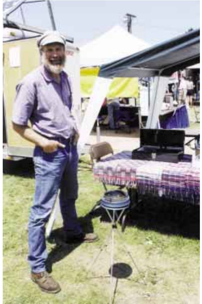
Cliff Millsapps demonstrates how the Solar Pathfinder can evaluate a site's solar potential.
