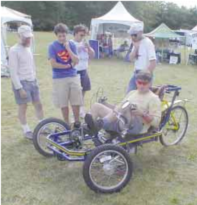
Josh Kerson with his prototype Spincycle, a solar-charged, human hybrid, electric recumbent tricycle. The pedals drive a generator to charge a battery. A small motor powers the rear wheel.
