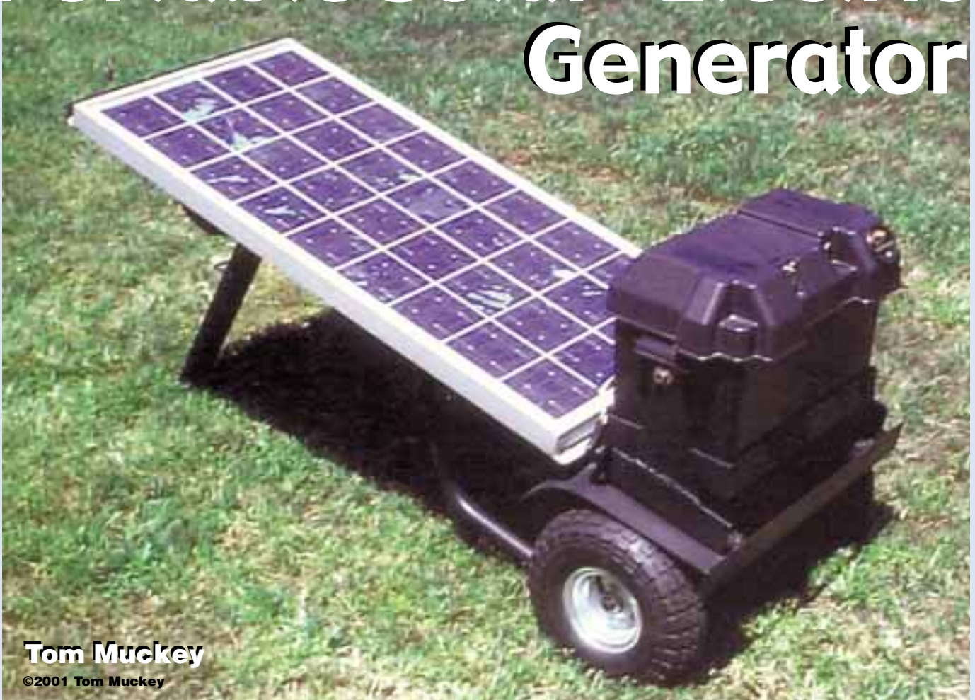
Tom Muckey's homemade, solar-electric generator on wheels solved his outbuilding's power problem.
