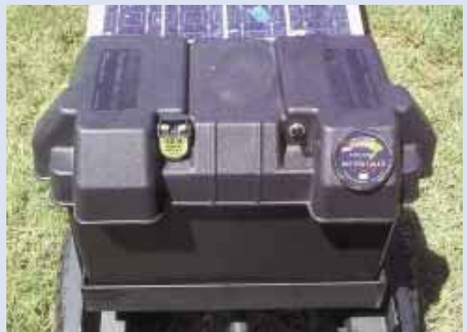
The front of the weather-resistant battery case, showing from left to right: 12 volt outlet, test switch, and battery meter.
