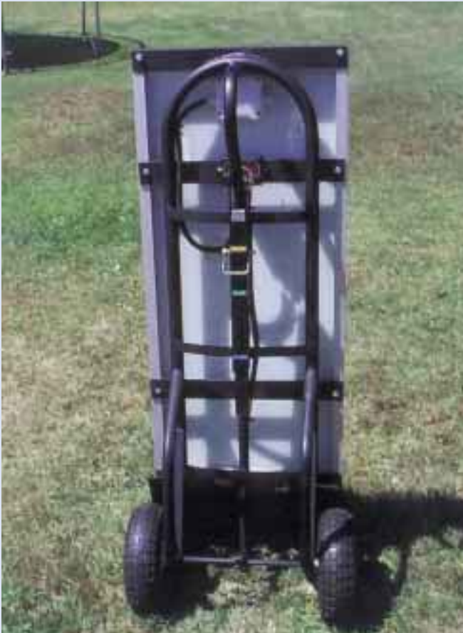
The back side of the modified hand truck. Note the seasonal tilt indicators marked with yellow, green and blue.
