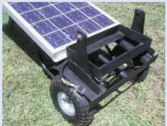
This homemade battery cradle keeps the flooded lead-acid battery level so electrolyte doesn't spill.
