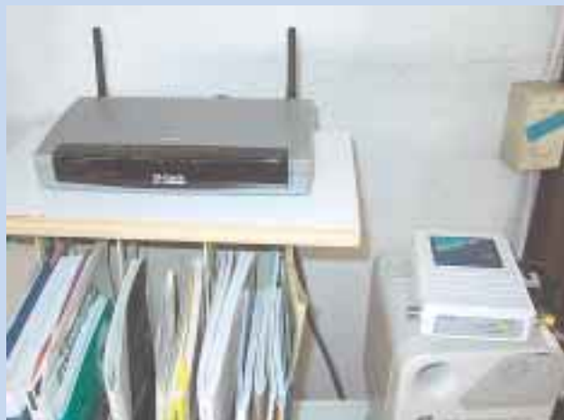
The D-Link router and the radio transceiver allow completely wireless Internet use.
