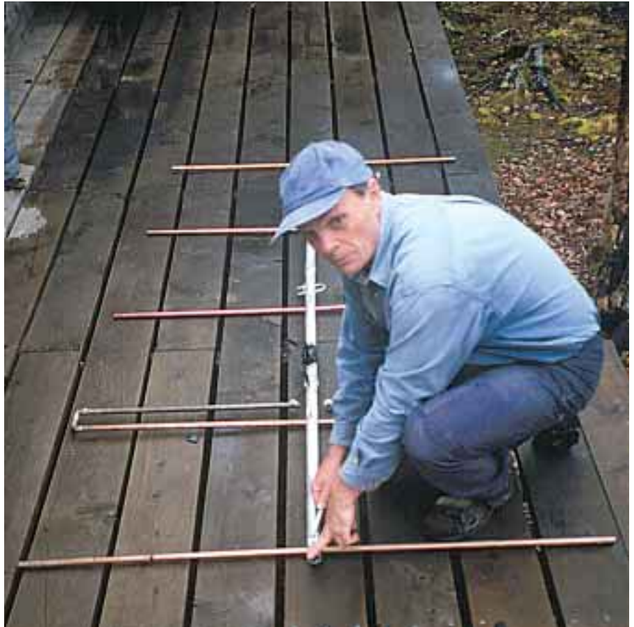
Author Bill Layman assembles a custom-tuned, five-element Yagi, FM antenna from salvaged parts.
