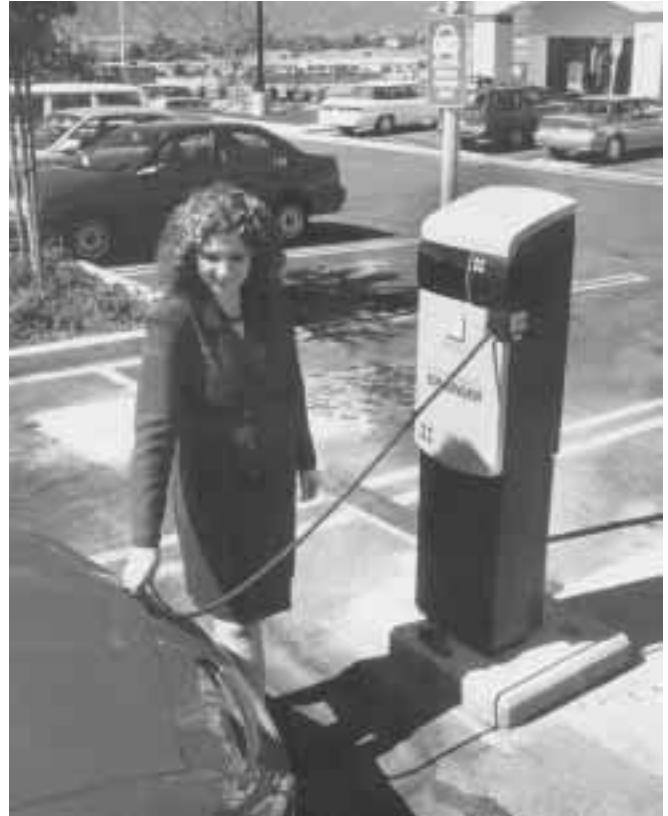
A GM EV-1 gets a charge through the MagneCharge's inductive connector.
