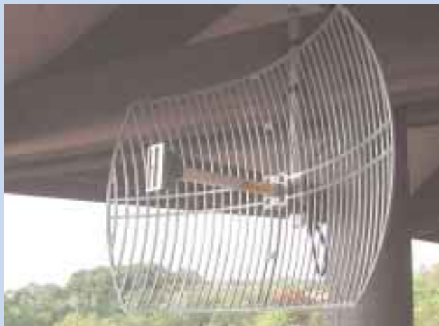
The radio system's receiving dish. The wireless Internet system only draws 1 to 2 watts total.
