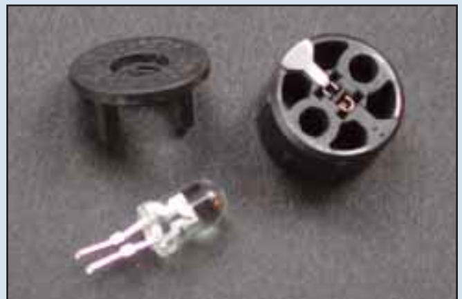
A closer look at the LED, bulb holder, and base.
