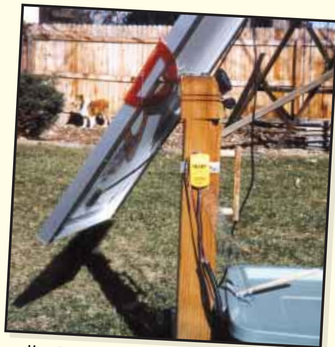
Horatio's mechanism adjusts angle and azimuth. Notice the protractor for determining tilt angle.
