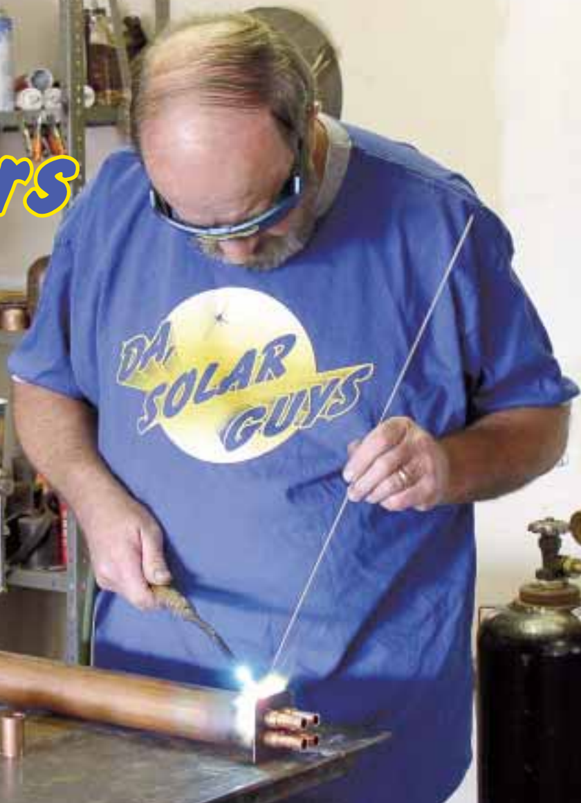
Don Keefe of AAA Solar brazes a double-wall, shell and tube, heat exchanger.
