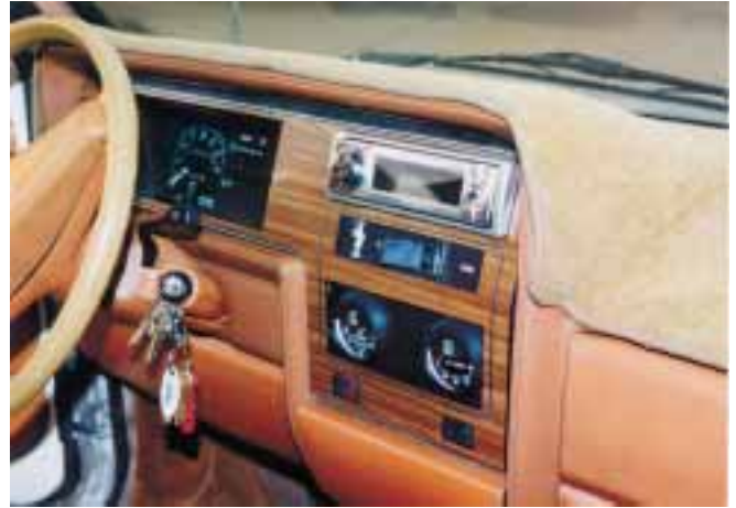
The truck's dash houses an ammeter for real-time feedback, a circuit breaker just in case of an electrical emergency, and a stereo so Joe and Emily can rock out, together.
