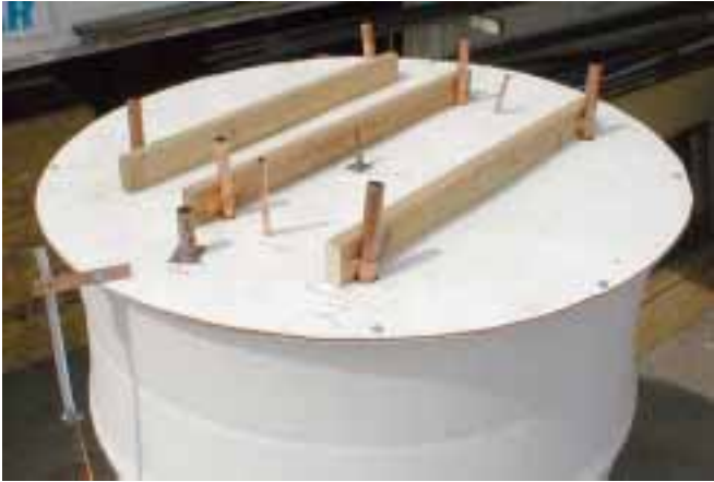
A 900 gallon tank with coils for glycol, DHW, space heat, and swimming pool.
